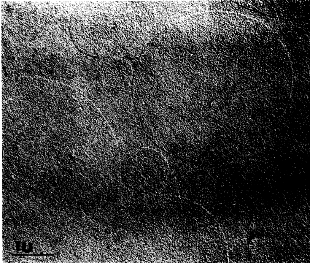
Fig. 15. Condensed phases in stearic acid film on water surface are shown as circular areas. Electron micrograph by H. E. Ries, Jr. (1961).
