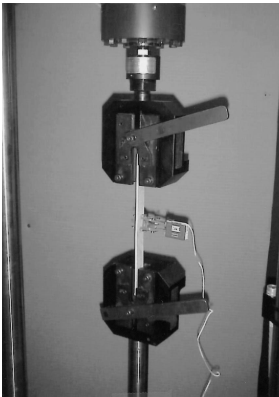
FIG. 3. The experimental setup for static MOE measurements parallel to the grain.
