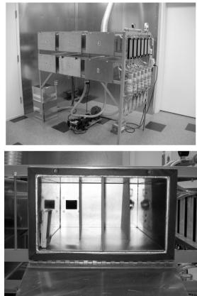
Figure 2. Typical small-chamber testing facility at a California Air Resources Board-approved third-party certifier (top photo: bank of six small chambers at the Composite Panel Association testing facility in Leesburg, VA; bottom photo: interior of small chamber with samples loaded for testing).
