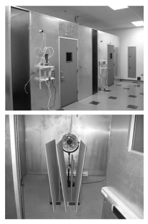
Figure 1. Typical large-chamber testing facility at a California Air Resources Board-approved third-party certifier (top photo: exterior of large chambers with air sampling apparatus shown at the Composite Panel Association testing facility in Leesburg, VA; bottom photo: interior of large chamber with samples loaded for testing).
