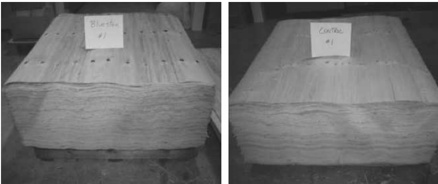
FIGURE 1. Dried MPB and control SPF veneer sheets sampled from a plywood mill.
