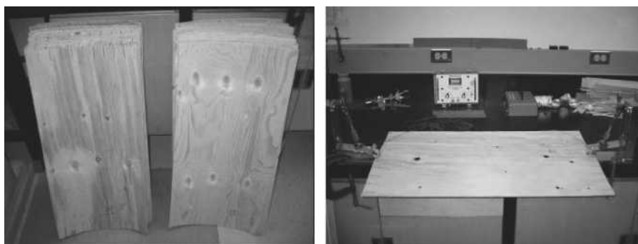
FIGURE 2. Pilot plant veneer stress wave testing.
