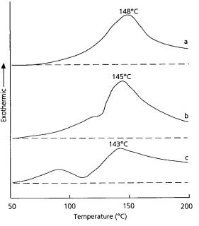
FIG. 3. DSC thermograms of reactions of phenolic adhesive mixture (a) alone, (b) with CCA-treated (9.6 kg/m<sup>3</sup>) southern pine in a 5:1 (adhesive-to-wood) weight-ratio, and (c) with CCA-treated (9.6 kg/m<sup>3</sup>) southern pine in a 2:1 (adhesive-to-wood) weight-ratio.
