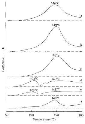
FIG. 1. DSC thermograms of reactions of phenolformaldehyde resin (a) alone, (b) with NaOH, and (c) with adhesive mixture constituents. Thermograms of adhesive mixture constituents are shown for (d) Co-Cob and wheat flour with NaOH and water, (e) Co-Cob with NaOH and water, and (f) wheat flour with NaOH and water.
