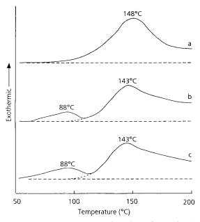
FIG. 2. DSC thermograms of reactions of phenolic adhesive mixture (a) alone, (b) with CCA-treated (9.6 kg/m<sup>3</sup>) southern pine in a 2:1 (adhesive-to-wood) weight-ratio, and (c) with untreated southern pine in a 2:1 (adhesive-to-wood) weight-ratio.
