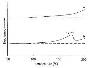
FIG. 4. DSC thermograms of reactions of (a) untreated southern pine and (b) CCA-treated (9.6 kg/m<sup>3</sup>) southern pine.
