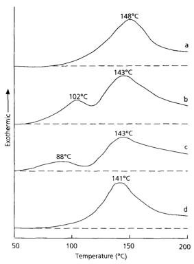
FIG. 5. DSC thermograms of reactions of phenolic adhesive mixture (a) alone, (b) with a 1.75% solution of CCA preservative, (c) with CCA-treated (9.6 kg/m<sup>3</sup>) southern pine in a 2:1 (adhesive-to-wood) weight-ratio, and (d) with a NaOH-precipitated and dried CCA preservative.
