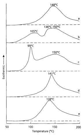
FIG. 6. DSC thermograms of reactions of phenolic adhesive mixture (a) alone; or with 1.87% weight of (b) total  $Cr^{+6}$ ,  $Cu^{+2}$ , and  $As^{+5}$  in solution of CCA preservative; (c)  $Cr^{+6}$  in solution of chromium trioxide (CrO<sub>3</sub>); (d)  $Cu^{+2}$  in solution of cupric chloride (CuCl<sub>2</sub>); and (e)  $As^{+5}$  in solution of arsenic pentoxide ( $As_2O_5$ ).
