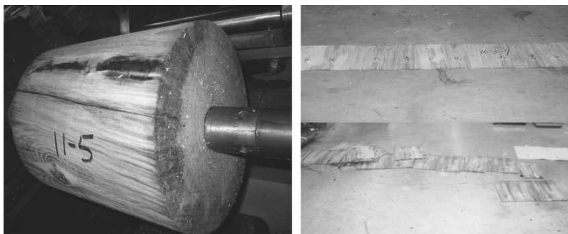
FIGURE 4. Peeling MPB blocks with a pilot plant 38-cm mini-lathe.
