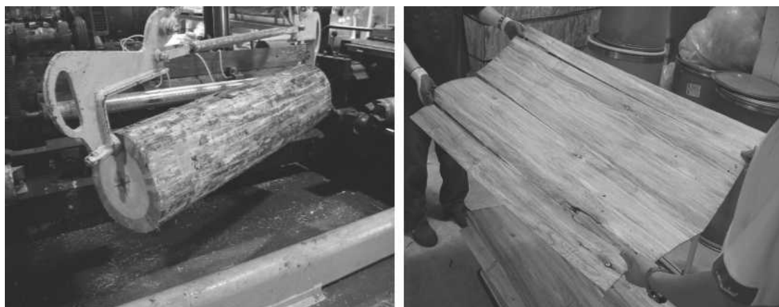
FIGURE 5. Pilot plant scale-up peeling test with a 1.2-m lathe.
