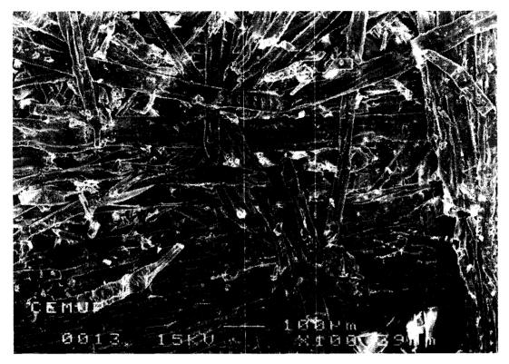
Fig. 2. Failure surface exposed of an MDF sample subjected to an internal bond test, obtained using SEM (magnification is  $\times$  100).
