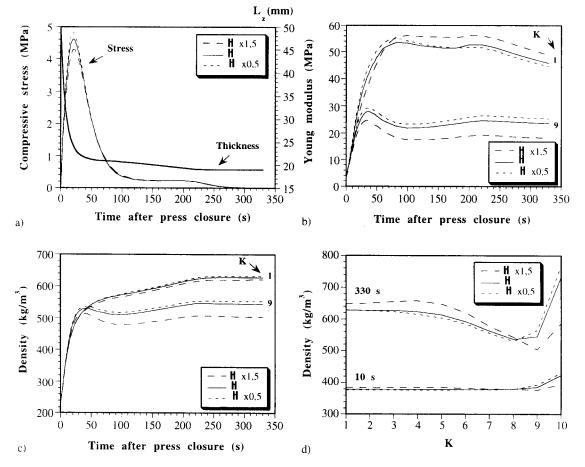
FIG. 8. Effect of initial mattress moisture content; evolution of a) overall compressive stress; b) Young's modulus; and c) density with time after press closure for several positions in the vertical direction (numbered from K = 1-adjacent to board mid-plane to K = 10-adjacent to board surface); d) vertical profiles of density, along the zz axis, at the board mid-plane for different times after press closure.
