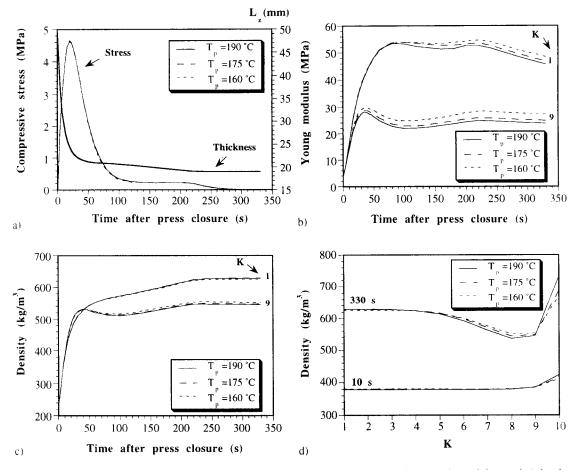
FIG. 7. Effect of platen temperature; evolution of a) overall compressive stress; b) Young's modulus; and c) density with time after press closure for several positions in the vertical direction (numbered from K = 1-adjacent to board mid-plane to K = 10-adjacent to board surface); d) vertical profiles of density, along the zz axis, at the board mid-plane for different times after press closure.
