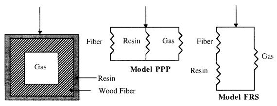
FIG. 4. Cell model and micromechanical models for MDF.
