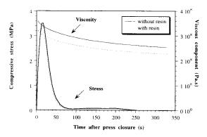
FIG. 9. Results for the viscous component of the composite estimated with and without resin: evolution of overall compressive stress with time after press closure.
