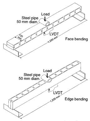
Fig. 5. Load application for center-point bending tests in face bending and edge bending orientations.
