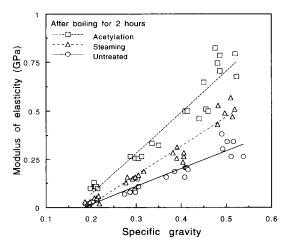
FIG. 4. Modulus of rupture of aspen fiberboards after 2 h in boiling water.
