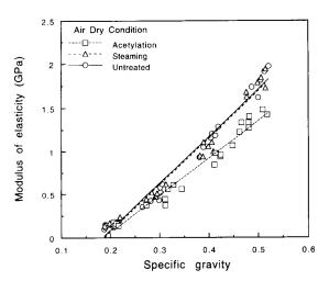
FIG. 1. Modulus of elasticity of aspen fiberboards at 60% RH and 20 C.
