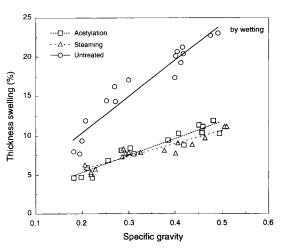
FIG. 6. Thickness swelling of aspen fiberboards after water soaking.
