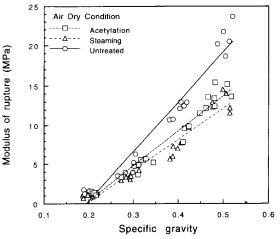
FIG. 2. Modulus of rupture of aspen fiberboards at 60% RH and 20 C.
