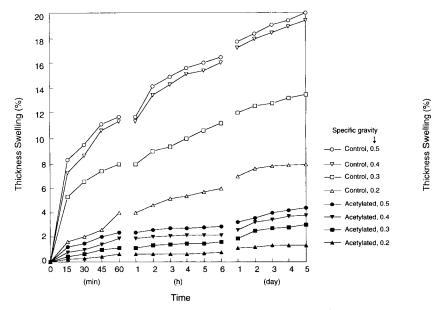
FIG. 8. Thickness swelling of untreated and acetylated aspen fiberboards in water.
