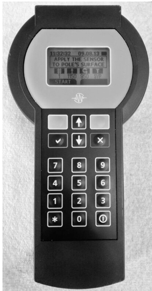
Figure 2. The PoleXpert device used to nondestructively evaluate in-service wood utility poles.
