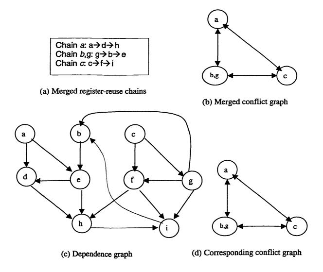
Figure 5.12 Dependence-conservative register-reuse chains
