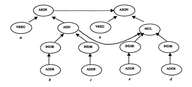
Figure 3.7 Adjustment of output dependence after register allocation
