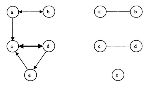
(a) Edge (c,d) is converted to a bidirectional edge
