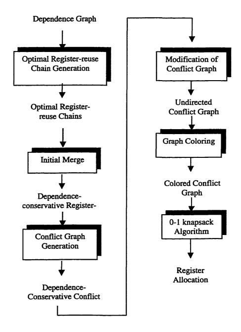
Figure 5.17 Complete procedure for register allocation
