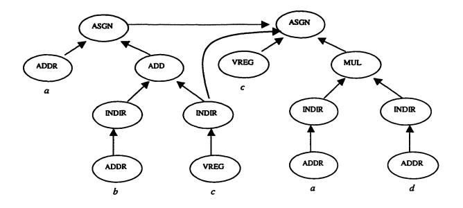
(a) Anti-dependence graph after a register is assigned to variable c
