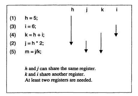
Figure 2.5 Effect of instruction scheduling on register allocation
