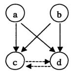
Figure 4.8 An example for additional dependence forcing simultaneous execution of c and d
