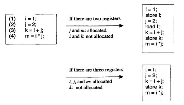
Figure 2.3 Example for register allocation
