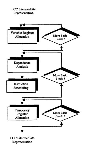
Figure 3.1 The structure of the new optimizing compiler
