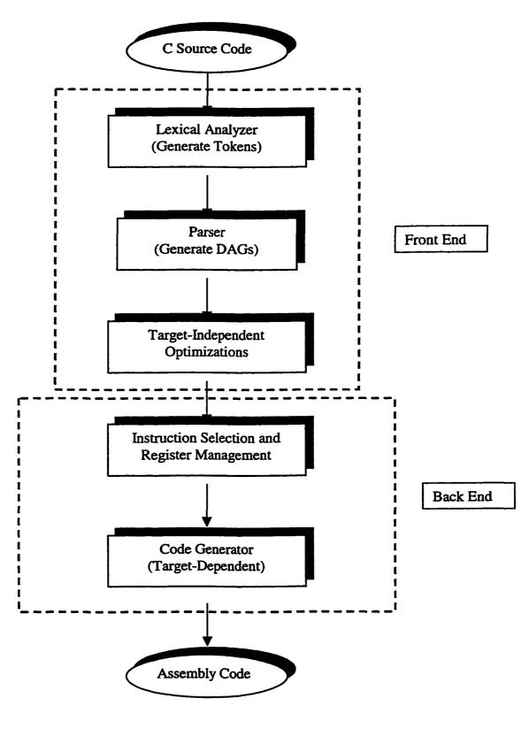
Figure 2.7 Structure of Local C Compiler (LCC)
