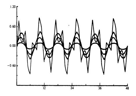
Fig.4.23 The fine grid residual is transferred to the coarse grid by full weighting. This figure shows the error after one relaxation sweep on the coarse grid residual equation, superimposed upon previous approximations.  $\|e\|_{\infty} = .977 \times 10^{-1}$ .
