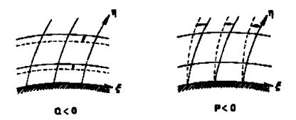
Fig.2.7 Effect of control function on coordinate lines.
