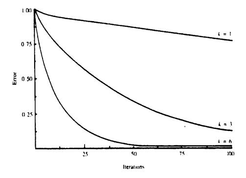
Fig.4.6 Regular Gauss-Seidel iteration applied to the one-dimensional model problem with N=64 and with initial guesses of  $v_1$ ,  $v_3$ , and  $v_6$ . The maximum norm of the error  $||e||_{\infty}$  is plotted against the iteration number for 100 iterations.
