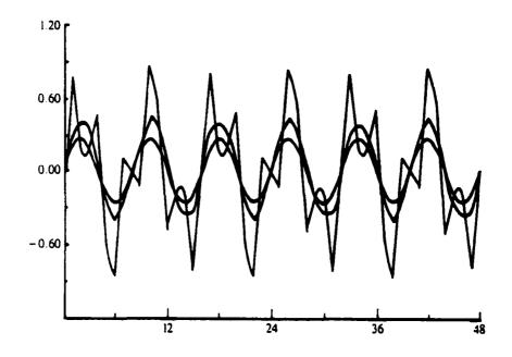
Fig.4.22 The error after three fine grid relaxation sweeps superimposed upon the previous iterates.  $||e||_{\infty} = .261$ .
