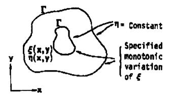
Fig.2.2 Boundary-conforming coordinate system.
