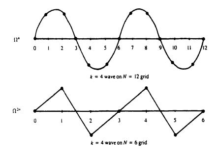
Fig.4.16 A wave with wavenumber k=4 on  $\Omega^{h}$  (N=12) is projected onto  $\Omega^{2h}$  (N=6). The coarser grid "sees" a wave with k =4 which is more oscillatory on the coarser grid than on the fine grid.
