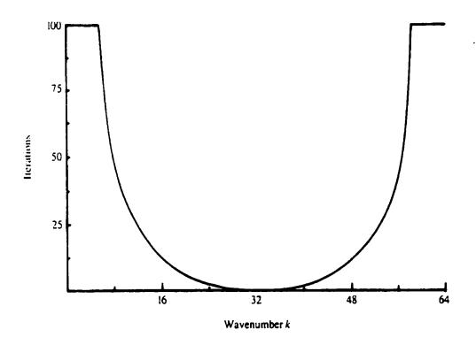
Fig.4.11 The weighted Jacobi method with w = 1 applied to the one-dimensional model problem with N=64. The initial guesses consist of the modes  $w_k$  for  $1 \le k \le 63$ . The graph shows the number of iterations required to reduce the norm of the initial error by a factor of 100 for each  $w_k$ .
