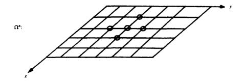
Fig.4.2 Two-dimensional grid on the unit square. The circled points show the unknowns that are related at a typical grid point by the discrete equations.
