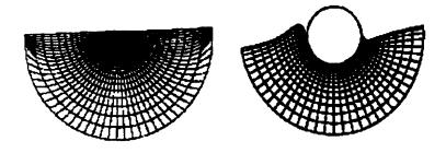
Fig.2.11 Effect of control function on boundary point distribution.
