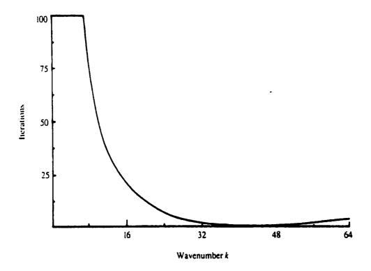
Fig.4.12 The weighted Jacobi method with w = 2/3 applied to the one-dimensional model problem with N=64. The initial guesses consist of the modes  $w_k$  for  $1 \le k \le 63$ . The graph shows the number of iterations required to reduce the norm of the initial error by a factor of 100 for each  $w_k$ . Note that for w = 2/3 the damping is the strongest for the oscillatory modes  $(32 \le k \le 63)$ .
