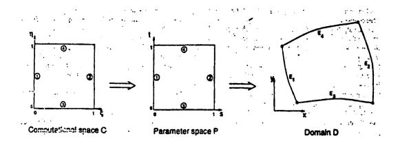
Fig.2.12 Transformation from computational  $(\xi, \eta)$  space to a domain D in Cartesian (x, y) space.
