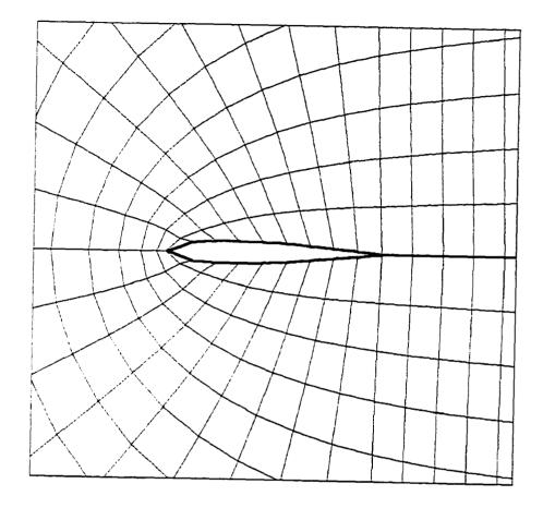
Fig.3.3. Grid generated using fourth-order compact finite difference schemes.
