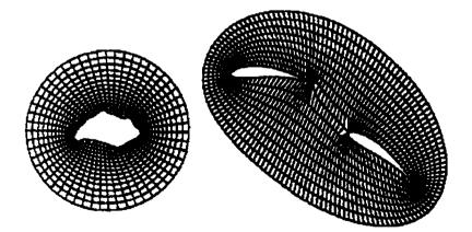
Fig.2.6 Examples of concave and convex boundaries.
