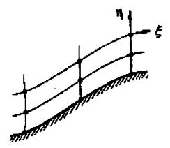
Fig.2.1 The curvilinear coordinate system.
