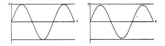
Fig.4.13 The weighted Jacobi method with w = 2/3 applied to the one-dimensional model problem with N=64 and an initial guess consisting of  $w_3$ . The figure shows the approximation after one iteration (on the left) and after ten iterations (on the right).
