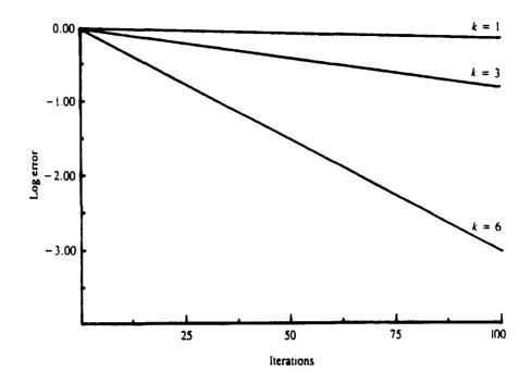
Fig.4.8 The weighted Jacobi method with w = 2/3 applied to the one-dimensional model problem with N=64 and with initial guesses consisting of  $v_1$ ,  $v_2$  and  $v_6$ . The log of  $||e||_{\infty}$  is plotted against the iteration number for 100 iterations.
