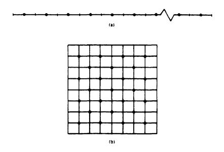
Fig.4.3 (a) One-dimensional and (b) two-dimensional grids showing the red points (unmarked) and black points (•) for the red-black relaxation.
