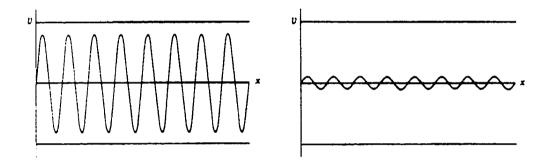
Fig.4.14 The weighted Jacobi method with w = 2/3 applied to the one-dimensional model problem with N=64 and an initial guess consisting of  $w_{16}$ . The figure shows the approximation after one iteration (on the left) and after ten iterations (on the right).
