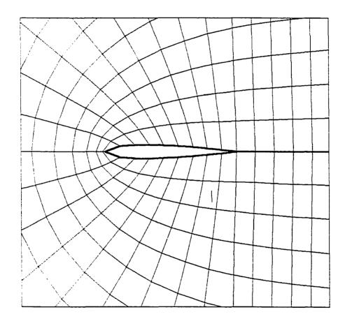
Fig.3.2. Grid generated using fourth-order standard finite difference scheme.
