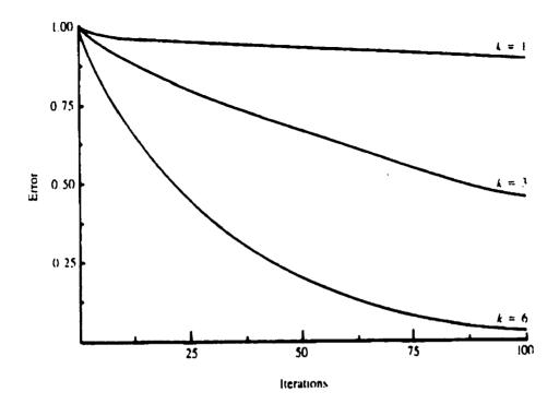
Fig.4.5 The weighted Jacobi method with w = 2/3 applied to the one-dimensional model problem with N=64 and with initial guesses of  $v_1$ ,  $v_3$ , and  $v_6$ . The maximum norm of the error  $||e||_{\infty}$  is plotted against the iteration number for 100 iterations.
