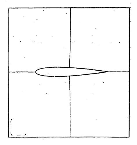
Fig.2.14 Domain boundaries near NACA0012 airfoil.
