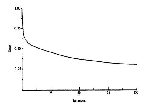
Fig.4.9 The weighted Jacobi method with w = 2/3 applied to the one-dimensional model problem with N = 64 and with initial guesses consisting of  $\frac{1}{3} \left[ \sin\left(\frac{j\pi}{N}\right) + \sin\left(\frac{6j\pi}{N}\right) + \sin\left(\frac{32j\pi}{N}\right) \right]$ . The maximum norm of the error ||e|| is plotted against the iteration number for 100 iterations.
