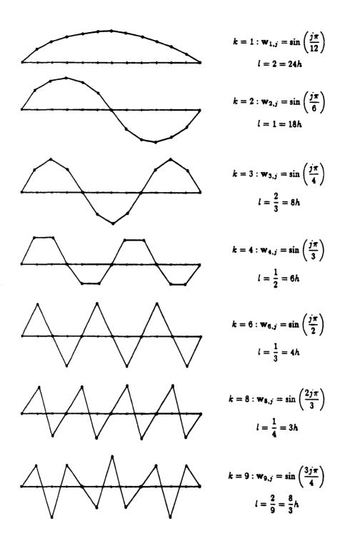
Fig.4.10 Graphs of the Fourier modes of A on a grid with N=12. Modes with wavenumbers k = 1,2,3,4,6,8,9 are shown. The wavelength of the kth mode is l = 24h/k.
