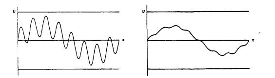
Fig.4.15 The weighted Jacobi method with w = 2/3 applied to the one-dimensional model problem with N=64 and an initial guess consisting of a combination of  $w_2$  and  $w_{16}$ . The figure shows the approximation after one iteration (on the left) and after ten iterations (on the right).
