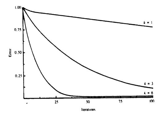
Fig.4.7 Red-black Gauss-Seidel iteration applied to the one-dimensional model problem with N=64 and with initial guesses of  $v_1$ ,  $v_3$ , and  $v_6$ . The maximum norm of the error  $||e||_{r}$  is plotted against the iteration number for 100 iterations.
