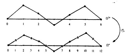
Fig.4.17 Interpolation of a vector on the coarse grid  $\Omega^{2h}$  to the fine grid  $\Omega^{h}$ .
