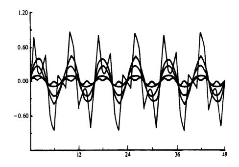
Fig.4.24 The error after relaxation sweeps on the coarse grid residual equation superimposed upon previous approximations.  $\|e\|_{rel} = .591 \times 10 - 1$
