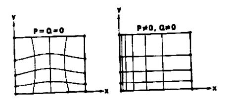
Fig.2.10 Effect of boundary point distribution,
