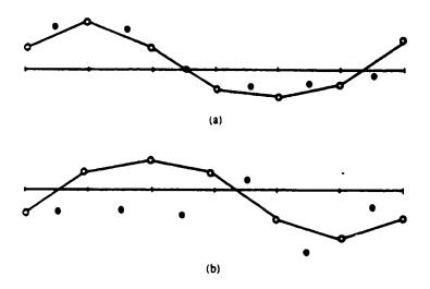
Fig.4.18 (a) If the exact error on  $\Omega^h$  (indicated by ° and •) is smooth, an interpolant of the coarse grid approximation  $e^{2h}$  (indicated by °) should give a good representation of the exact error. (b) If the exact error on  $\Omega^h$  (indicated by ° and •) is oscillatory, an interpolant of the coarse grid approximation  $e^{2h}$  (indicated by °) may give poor representation of the exact error.
