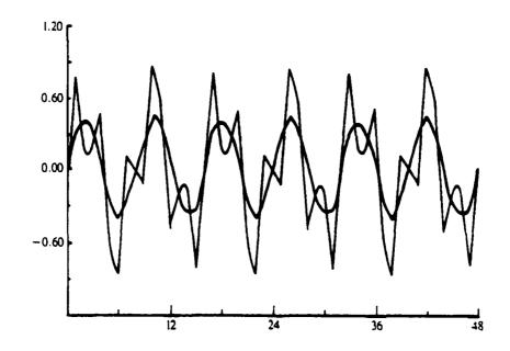
Fig.4.21 The approximation (and error) after one fine grid relaxation sweep superimposed upon the initial guess.  $\|e\| = .430$ .
