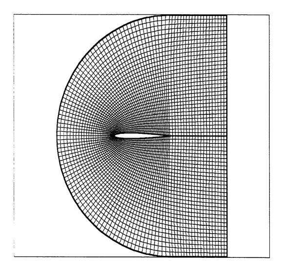
Fig.4.32 Grid generated near an airfoil.
