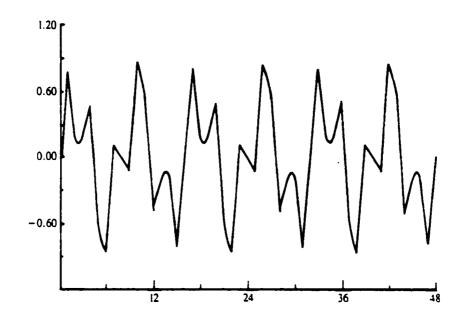
Fig.4.20 The initial guess  $v_j = 1/2 \left[ \sin\left(\frac{12j\pi}{N}\right) + \sin\left(\frac{30j\pi}{N}\right) \right]$  with N = 48 for a coarse grid correction scheme applied with the weighted Jacobi iteration (w = 2/3).  $||e||_{x} = 1.000$ .
