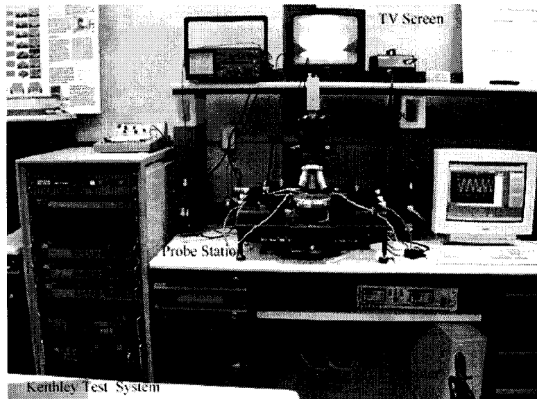
Figure 3-4 Schematic diagram of set-up for I-V and C-V measurement
