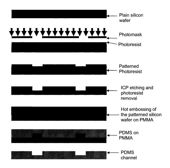
Figure 3.1. Microchannel formation through lithography, hot embossing and softlithography.
