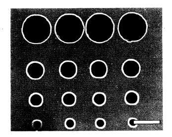
Figure 5.2. SEM image of a silicon substrate with gradient opening arrays, scale bar is 200  $\mu$ m.
