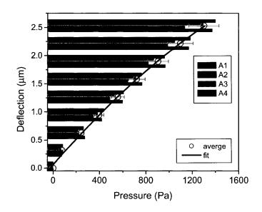
Figure 5.6. Four independent deflection-pressure sets of data (columns) obtained simultaneously for freely suspended nanomembranes with identical diameters along with the average behavior (solid line). The labels correspond to the membranes over different openings, as shown in Figure 5.4.
