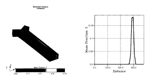
Figure 3.7. Simulation of the condition where the flow rate in the left inlet is five times the flow rate of the inlet on the right.
