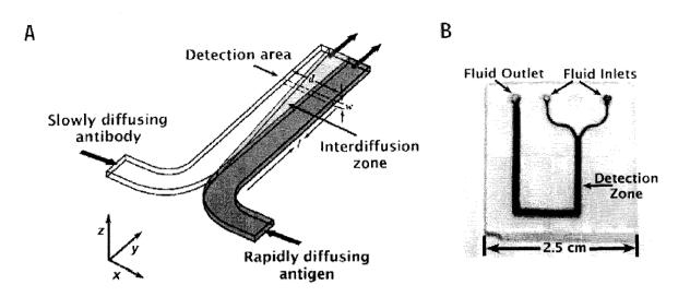
Figure 2.4. (a) Schematic of a diffusion immunoassay in a T-sensor and (b) a microfluidic device used for testing the immunoassay<sup>15</sup>.
