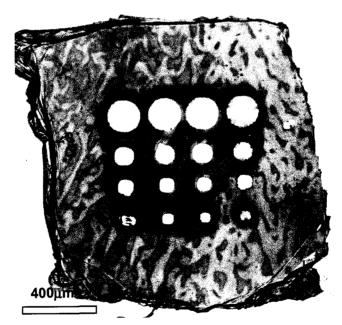
Figure 5.3. Optical image of the of  $4 \times 4$  array covered with LbL film.
