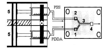
Figure 3.3. Schematic illustration of the laminar flow pattering experimental setup.
