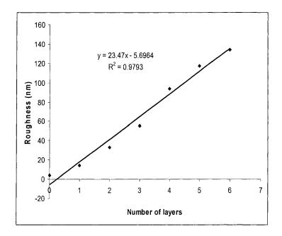
Figure 8.3. Change in surface roughness TiO<sub>2</sub> layers as a function of layer number.
