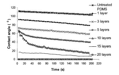
Figure 6.6. Water contact angle measurements on PDMS with the deposition of different number of layers of TiO<sub>2</sub>.
