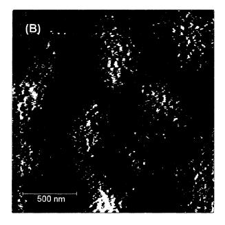
Figure 4.10. Confocal fluorescence (a) and atomic force microscopy (b) images of the PDDA/BSA micropattern. PDDA was labeled with FITC. Inlet flow rate was 0.01 mL•min-1 in both inlet channels; initial concentration of PDDA and BSA 0.1 mg•mL-1.
