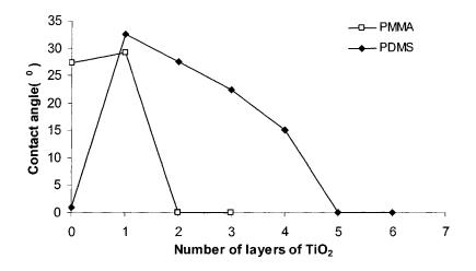
Figure 6.8. Water contact angle of PMMA and PDMS substrates after coating with different number of PSS/TiO<sub>2</sub> bilayers with plasma treatment of the substrates.
