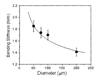
Figure 5.9. The bending rigidity of the nanomembranes as a function of the membrane diameter and the theoretical prediction of elastic membrane deformation (solid line).
