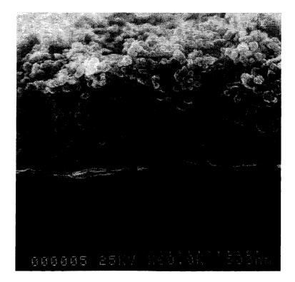
Figure 6.2. Scanning electron micrograph of  $(PDDA/PSS)_3 + (TiO_2/PSS)$  multilayer cross-section on a silver electrode. The particle diameter is ca 21 nm (Hitachi S-900 SEM operating at 25 kV; the sample is coated with 2 nm of Pt).
