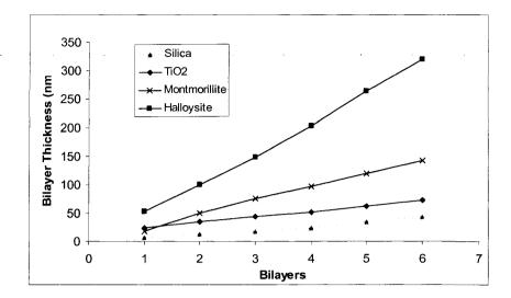
Figure 7.1. Thickness of the nanoparticle thin films measured using quartz resonators.
