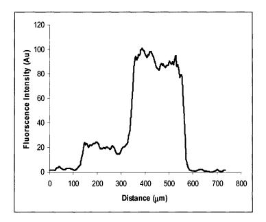
Figure 4.13. The line scan as a function of distance across the channel.
