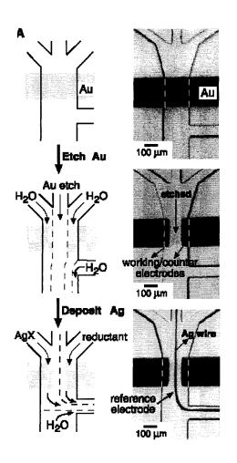
Figure 2.2. Etching of siliver and gold and the fabrication of complex electrical circuitry contained inside a microchannel<sup>9</sup>.
