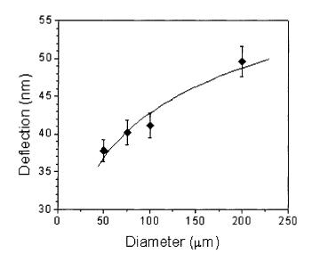
Figure 5.8. The deflection of nanomembranes with different diameters tested with the colloidal AFM probe under the applied force of 70 nN as a function of the membrane diameter.
