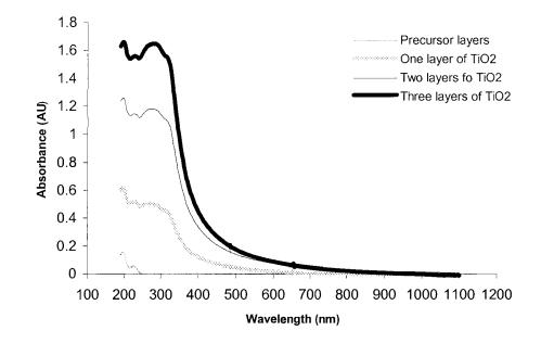
Figure 6.3. UV-vis absorbance with increasing number of layers of TiO<sub>2</sub>.
