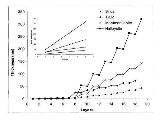
Figure 8.1. Change in thickness of the deposited nanoparticle films, monitored using quartz crystal microbalance. Inset shows the linear increase in thickness of the deposited layers.
