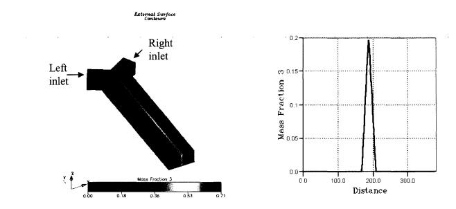
Figure 3.4. Left, Simulation results for equal flow rates in the left and right inlet channels and right, line graph of the mass fraction in the middle of the outlet channel.
