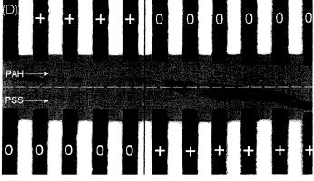
Figure 4.11. Effect of electric field on the position of the interpolyelectrolyte complex formed in the channel.
