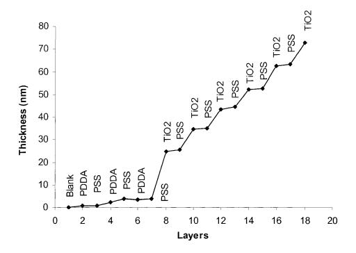
Figure 6.1. Film thickness as a function of deposited TiO<sub>2</sub> layers.
