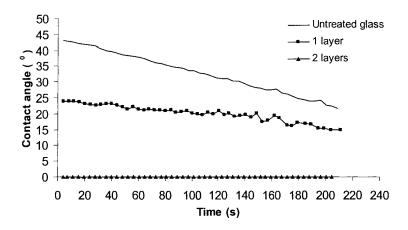
Figure 6.4. Water contact angle measurements on glass with the deposition of different number of layers of TiO<sub>2</sub>.
