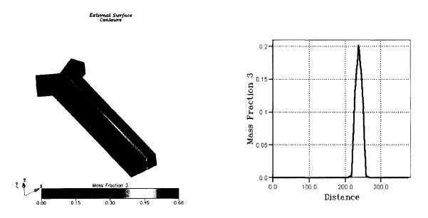
Figure 3.5. Simulation of the condition where the flow rate in the left inlet is 2 times the flow rate of the inlet on the right.
