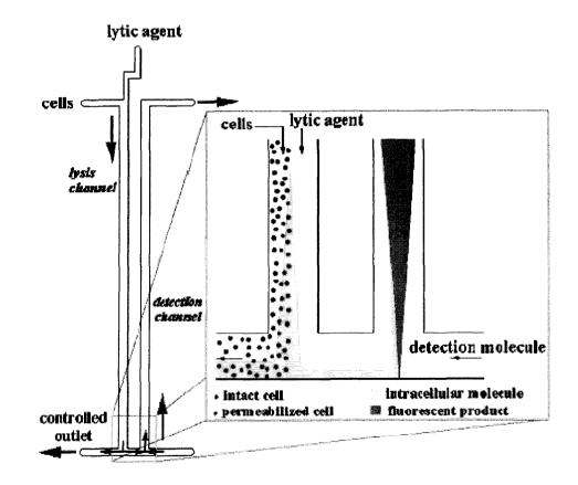
Figure 2.5. Schematic of microfluidic device for cell lysis and fractionation/detection of intercellular components<sup>35</sup>.
