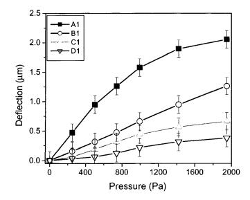
Figure 5.5. Deflection-pressure data for freely-suspended nanomembranes with different diameters.
