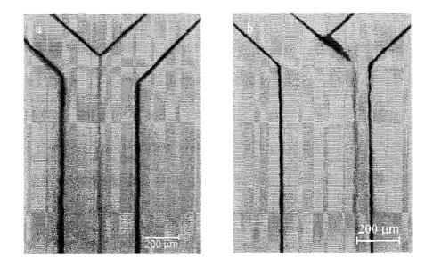
Figure 4.1. Optical micrographs of the formation of the polyelectrolyte complex inside the channel by varying the flow rates, (a) equal and (b) different flow rates.
