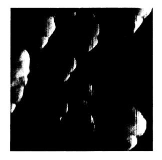
Figure 4.9. Atomic force microscopy image of PAH/citrate micropattern deposited onto glass support.
