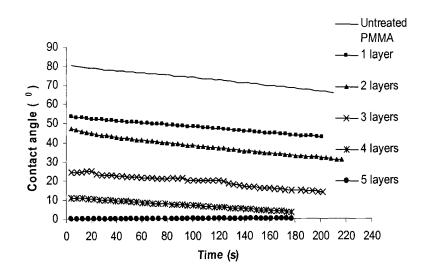
Figure 6.5. Water contact angle measurements on PMMA with the deposition of different number of layers of TiO<sub>2</sub>.
