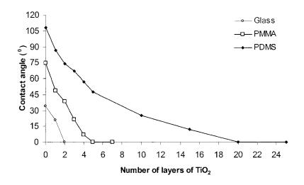
Figure 6.7. Water contact angle of glass, PMMA and PDMS substrates after coating with different number of PSS/TiO<sub>2</sub> bilayers without plasma treatment of the substrates.
