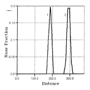
Figure 4.4. Numerical simulation of PDDA - PSS interaction inside channel microreactor.
