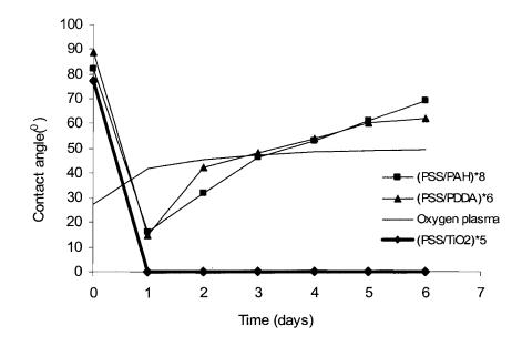
Figure 6.9. Change in water contact angle for various coatings on PMMA during storage; treatment was performed on the first day.
