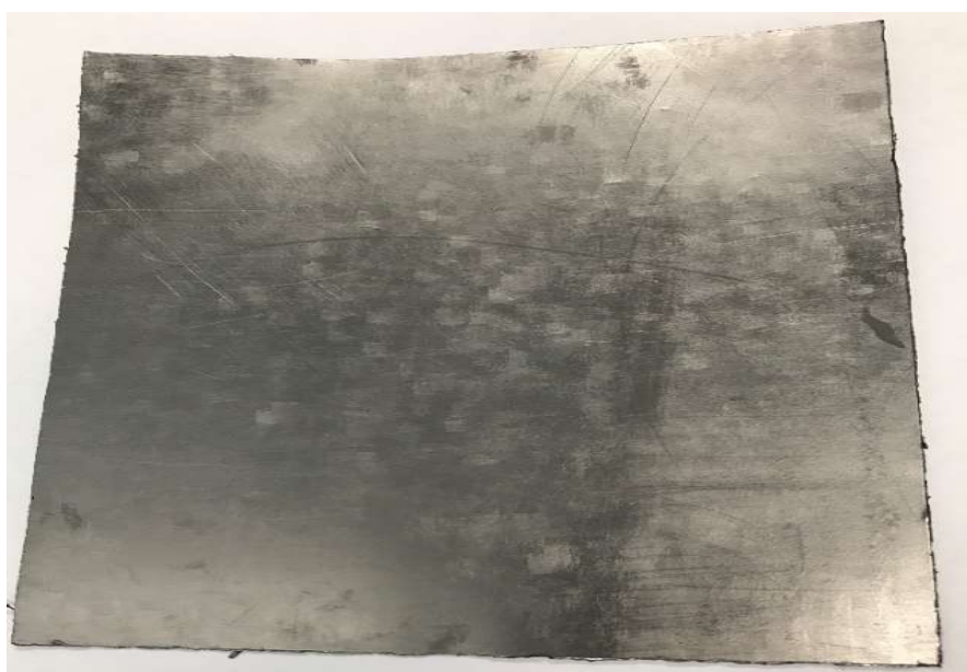
Figure 3-2: Flexible graphite sheet with no insert used as current collector.
