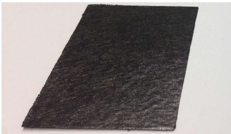
Figure 3-1: Carbon aerogel/fiber paper used as electrode in this study.
