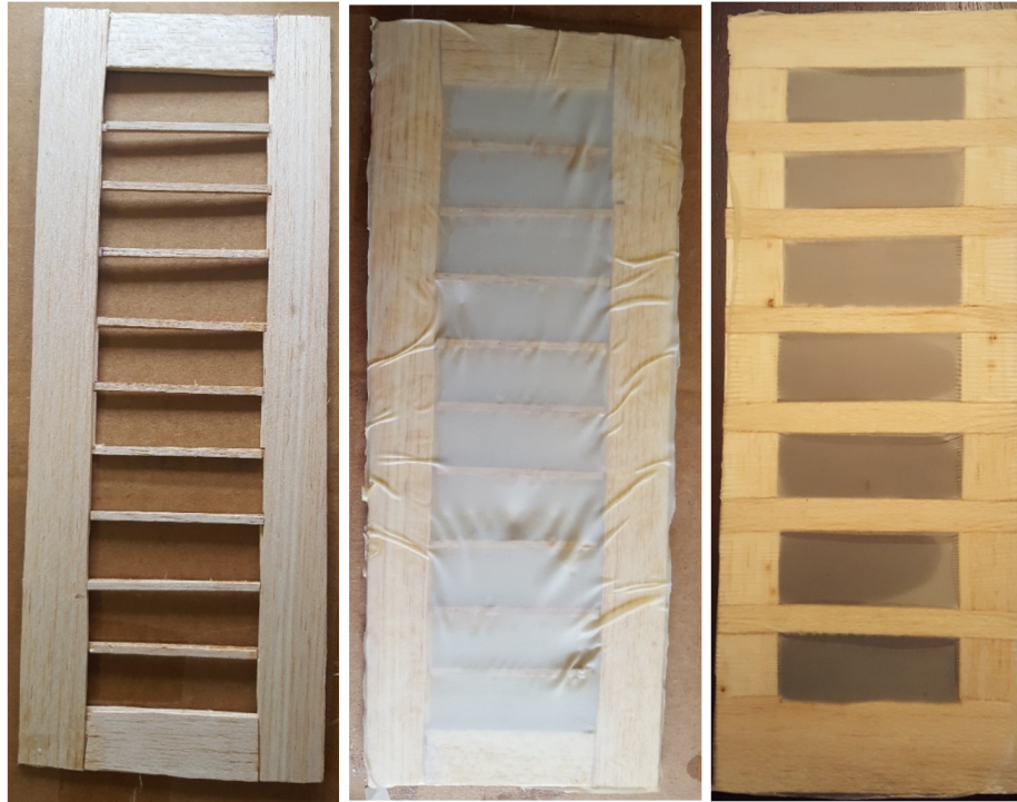
Figure 5.4: Effects of Applying Pretension to Latex
