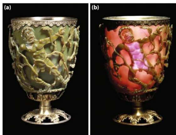
Figure 1-2: The Lycurgus cup appears (a) green when light is reflected off the surface of the cup, and (b) red when the light is transmitted through the cup [19].
