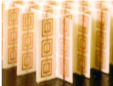
Figure 1-3: Bulk negative index materials with the unit cell consisting of SRR combined with the metallic wire [30].
