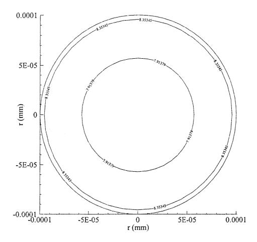
Figure 4.7 Contours of temperature distribution in the  $r\theta$  cross-section of the sphere subjected to symmetric pulse laser irradiation on the surface when t = 2.0 ps.
