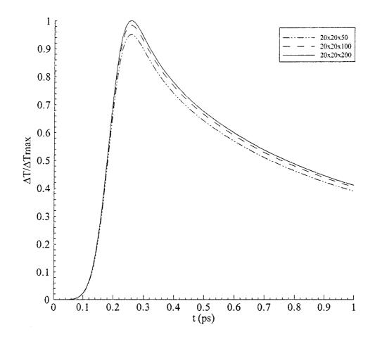
Figure 4.18 Temperature change with time at the top point of the sphere subjected to parallel pulse laser irradiation on a portion of the surface.
