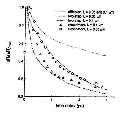
Figure 2.3 Transient reflectivity change at the front surface of gold films (thickness 0.05 and 0.1  $\mu m$ ) subjected to laser irradiation (pulse width 96 fs, energy flux 1 mJ/cm<sup>2</sup>) [Qiu 1992] [Brorson 1987].
