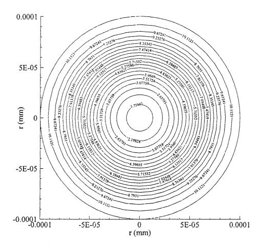
Figure 4.5 Contours of temperature distribution in the  $r\theta$  cross-section of the sphere subjected to symmetric pulse laser irradiation on the surface when t = 0.5 ps.
