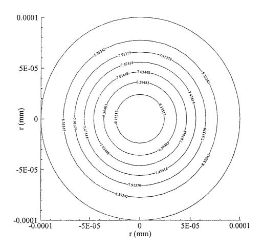
Figure 4.6 Contours of temperature distribution in the  $r\theta$  cross-section of the sphere subjected to symmetric pulse laser irradiation on the surface when t = 1.0 ps.
