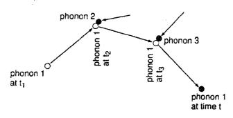
Figure 2.1 Energy transport through phonon collision.
