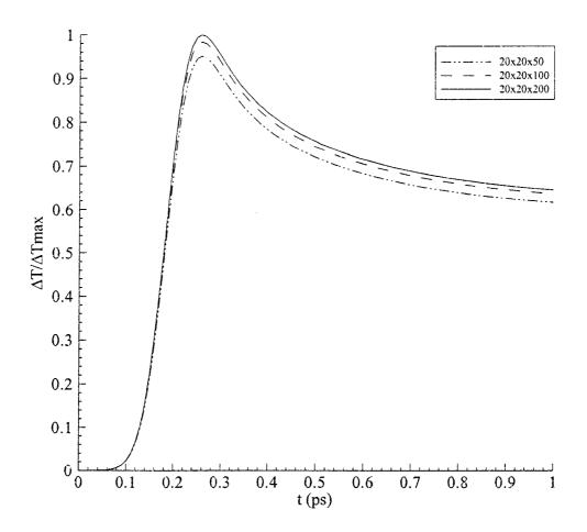
Figure 4.2 Temperature change with time at the surface of the sphere subjected to symmetric pulse laser irradiation.
