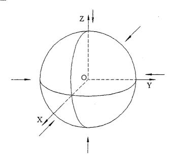
Figure 4.1 The gold sphere subjected to short-pulse laser irradiation on the surface  $(r = L, 0 \le \theta \le \pi, 0 \le \varphi \le 2\pi)$  symmetrically.
