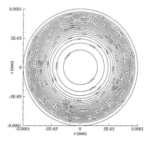
Figure 4.4 Contours of temperature distribution in the  $r\theta$  cross-section of the sphere subjected to symmetric pulse laser irradiation on the surface when t = 0.25 ps.
