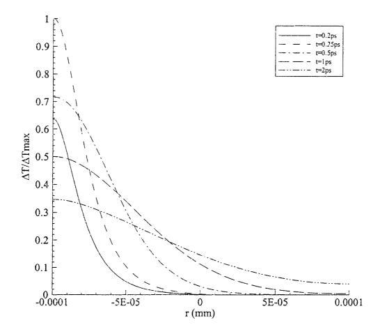
Figure 4.16 Temperature change along r-axis ( $\theta = 0$  and  $\pi$ ) of the sphere subjected to parallel pulse laser irradiation on the top half of the surface.
