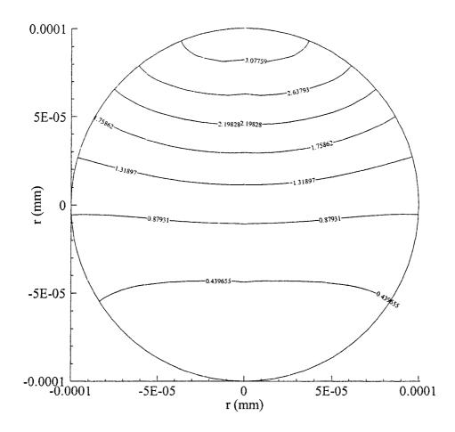
Figure 4.23 Contours of temperature distribution in the  $r\theta$  cross-section of the sphere subjected to parallel pulse laser irradiation on a portion of the surface when t = 2.0 ps.
