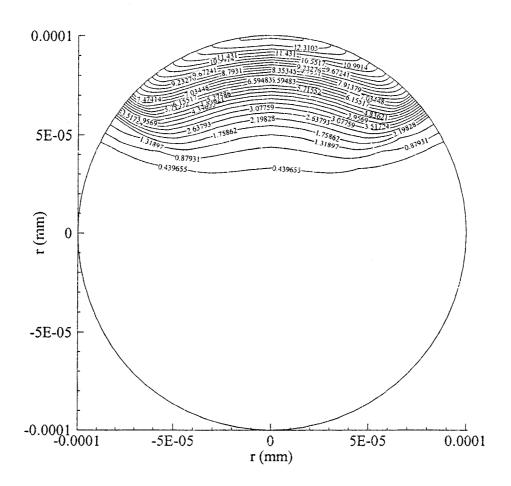
Figure 4.20 Contours of temperature distribution in the  $r\theta$  cross-section of the sphere subjected to parallel pulse laser irradiation on a portion of the surface when t = 0.25 ps.
