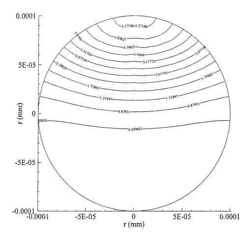
Figure 4.22 Contours of temperature distribution in the  $r\theta$  cross-section of the sphere subjected to parallel pulse laser irradiation on a portion of the surface when t = 1.0 ps.
