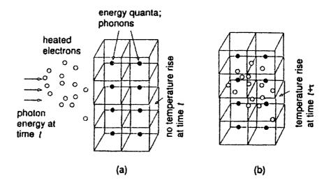
Figure 2.5 The finite time required for the phonon-electron interaction in microscale. (a) The first stage of electron-gas heating by phonons and (b) the second stage of metal lattice heating by phonon-electron interactions.
