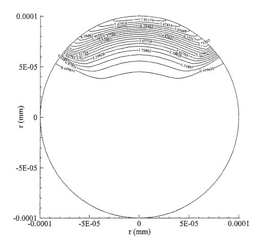
Figure 4.19 Contours of temperature distribution in the  $r\theta$  cross-section of the sphere subjected to parallel pulse laser irradiation on a portion of the surface when t = 0.2 ps.
