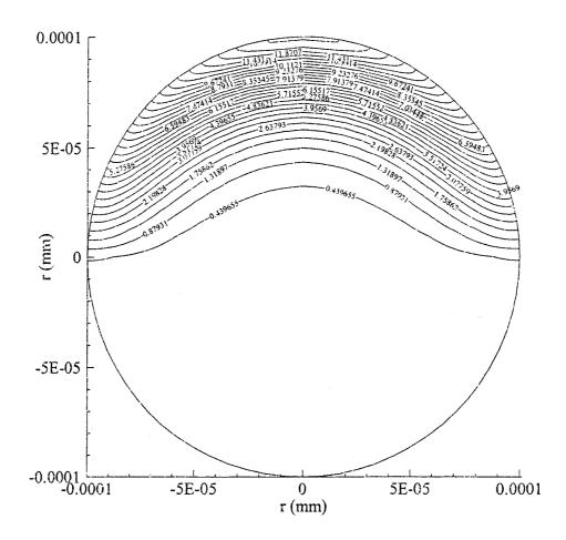
Figure 4.12 Contours of temperature distribution in the  $r\theta$  cross-section of the sphere subjected to parallel pulse laser irradiation on the top half of the surface when t = 0.25 ps.
