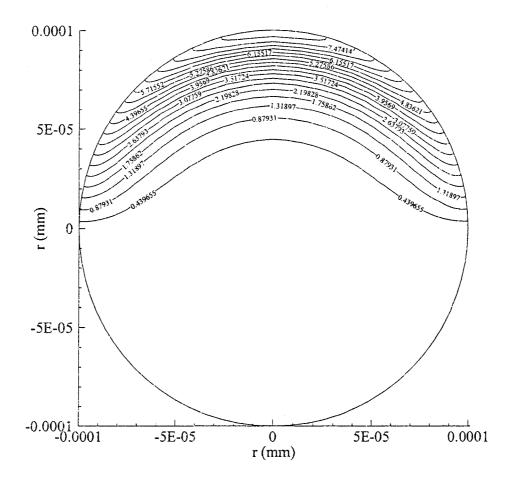
Figure 4.11 Contours of temperature distribution in the  $r\theta$  cross-section of the sphere subjected to parallel pulse laser irradiation on the top half of the surface when t = 0.2 ps.
