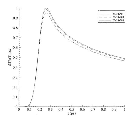
Figure 4.10 Temperature change with time at the top point of the sphere subjected to parallel pulse laser irradiation on the top half of the surface.
