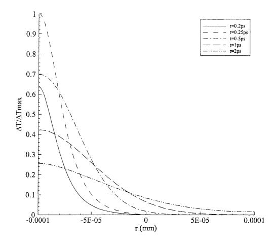
Figure 4.24 Temperature change along r-axis ( $\theta = 0$  and  $\pi$ ) of the sphere subjected to parallel pulse laser irradiation on a portion of the surface.
