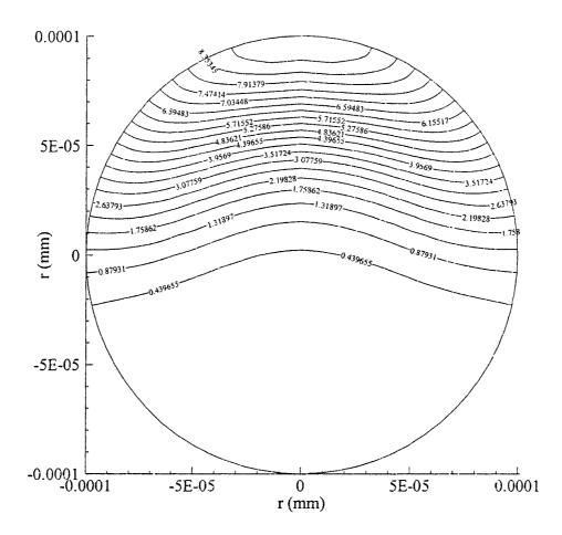
Figure 4.13 Contours of temperature distribution in the  $r\theta$  cross-section of the sphere subjected to parallel pulse laser irradiation on the top half of the surface when t = 0.5 ps.
