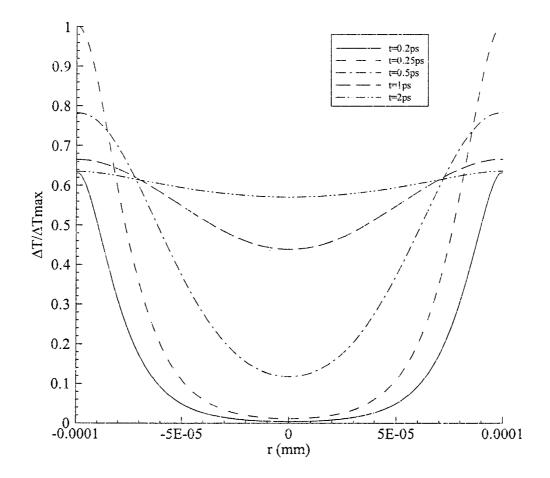
Figure 4.8 Temperature change along r-axis ( $\theta = 0$  and  $\pi$ ) of the sphere subjected to symmetric pulse laser irradiation on the surface.
