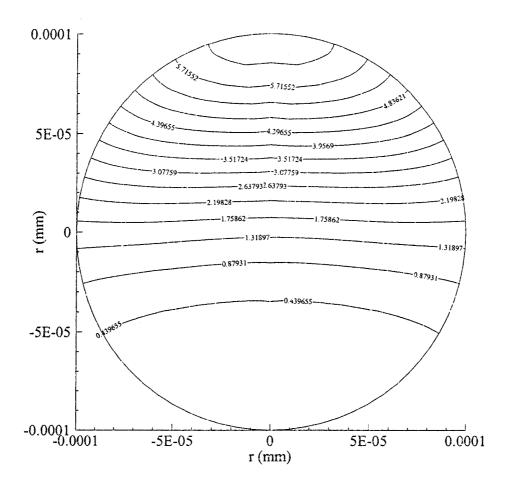
Figure 4.14 Contours of temperature distribution in the  $r\theta$  cross-section of the sphere subjected to parallel pulse laser irradiation on the top half of the surface when t = 1.0 ps.
