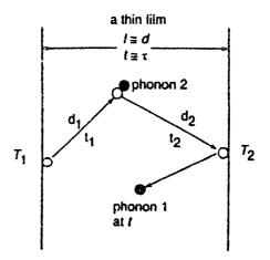
Figure 2.2 Phonon interaction in a thin film of the same order of magnitude as the mean free path, illustrating the challenge of the microscale effect in space to the concept of temperature gradient.
