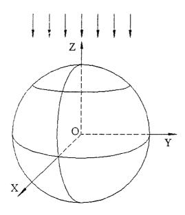
Figure 4.17 The gold sphere subjected to short-pulse laser irradiation on a portion of the surface  $(r = L, 0 \le \theta \le \frac{\pi}{4}, 0 \le \varphi \le 2\pi)$  in parallel.
