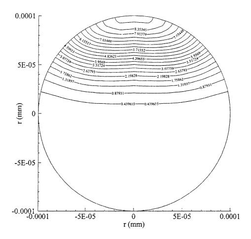
Figure 4.21 Contours of temperature distribution in the  $r\theta$  cross-section of the sphere subjected to parallel pulse laser irradiation on a portion of the surface when t = 0.5 ps.
