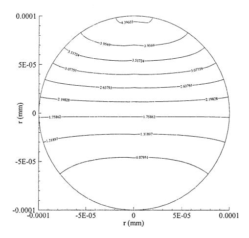
Figure 4.15 Contours of temperature distribution in the  $r\theta$  cross-section of the sphere subjected to parallel pulse laser irradiation on the top half of the surface when t = 2.0 ps.
