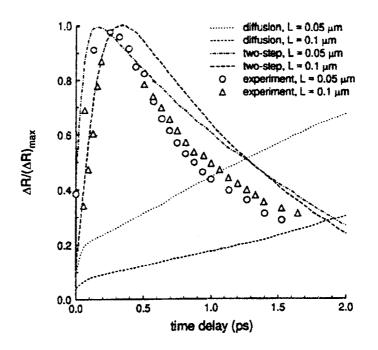
Figure 2.4 Transient reflectivity change at the rear surface of gold films (thickness 0.05 and 0.1  $\mu m$ ) subjected to laser irradiation (pulse width 96 fs, energy flux 1  $mJ/cm^2$ ). [Qiu 1992] [Brorson 1987].
