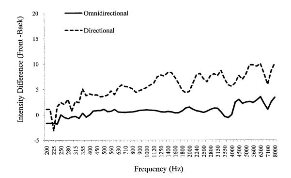
Figure 3 SPL difference between the front and back response for the omnidirectional and directional microphone conditions for all right ears. Note: Difference was calculated by subtracting front response from the back response.
