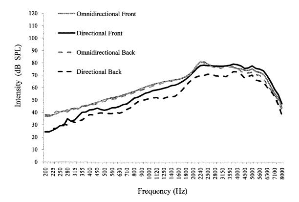
Figure 2 Average SPLs as a function of frequency for the omnidirectional and directional settings when measured from the front and back loudspeakers of the Verifit for 30 ears.
