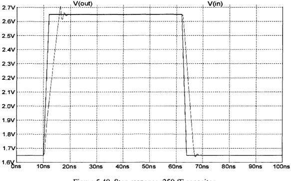
Figure 5.40 Step response, 250 fF capacitor.
