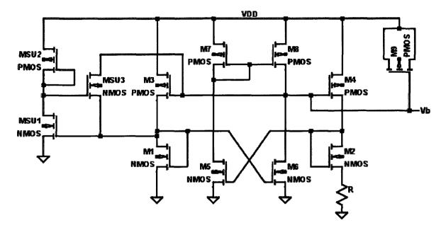
Figure 5.30 Current reference circuit with start-up circuit.
