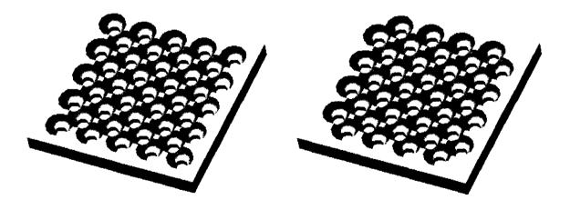
Figure 6.5 First stack layer design; layers are alternated as they are stacked.
