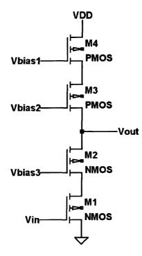
Figure 5.22 Cascode amplifier configuration.
