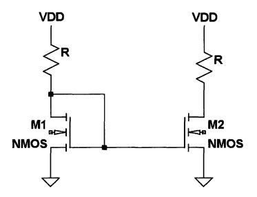
Figure 5.29 Basic current mirror with resistor loads.
