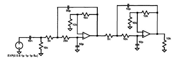
Figure 5.12 Schematic of 5<sup>th</sup> order filter.
