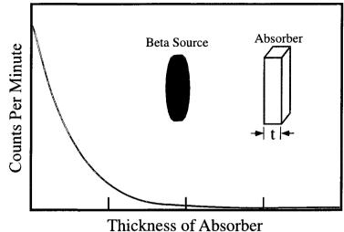
Figure 2.5 Range of beta particles.
