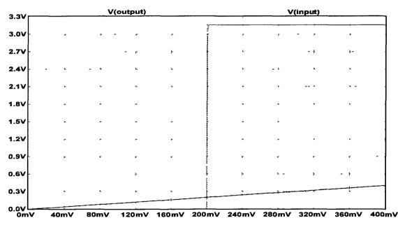
Figure 5.41 Comparator switching test at 200 mV.
