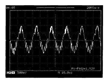
Figure 5.50 Inverting amplification of the 500 fF amplifier.
