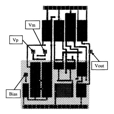
Figure 5.44 Comparator layout.
