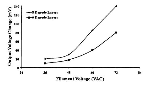
Figure 6.14 Voltage change versus filament voltage of the eight and six layer dynode stacks.
