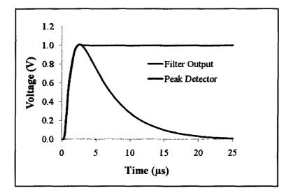
Figure 5.15 Peak detector output waveform.
