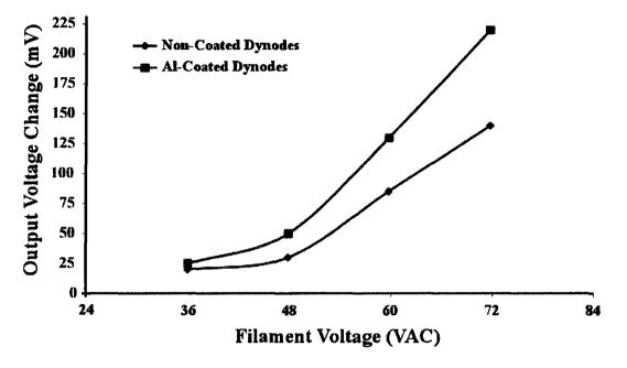
Figure 6.15 Voltage change versus filament voltage of the non-coated and Al-coated dynode stacks.
