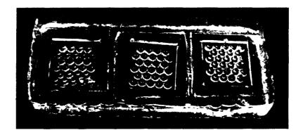
Figure 6.9 Reverse silicon mold of dynode master mold.
