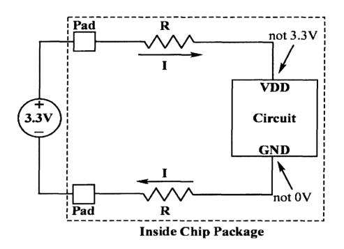
Figure 5.55 Under-sized power and ground traces become resistors in the circuit.
