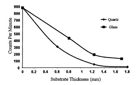
Figure 4.7 Glass and quartz absorption of beta particles as substrate thickness is increased.
