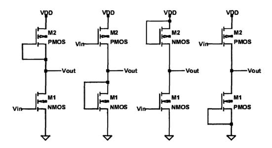
Figure 5.20 Four common-source amplifier configurations.
