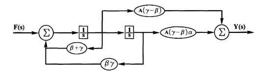
Figure 5.10 Canonical representation of the transfer function H(s).
