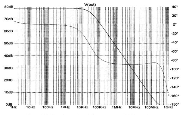
Figure 5.37 Open loop gain and phase response, 500 fF capacitor.
