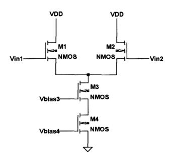
Figure 5.25 NMOS source-coupled differential pair.
