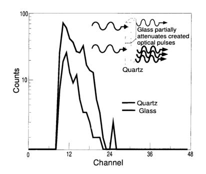
Figure 4.9 Glass and quartz have similar energy spectra allowing for glass or quartz to be used as the detecting medium.
