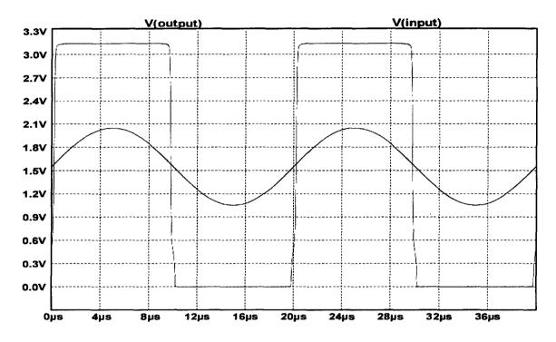
Figure 5.42 Transient response of the comparator.
