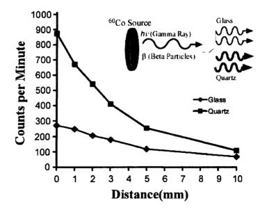
Figure 4.8 Testing the scintillator detectors with a gamma ray source for a function of counts per minute over varying distances.
