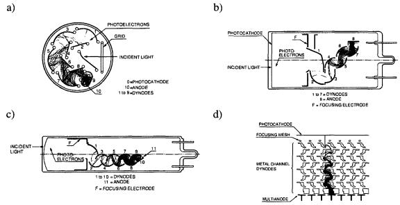
Figure 6.4 Photomultiplier tube dynode configurations [67].
