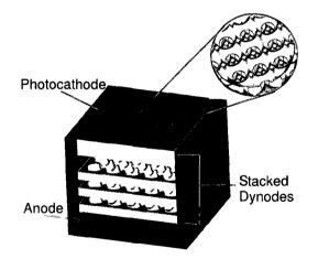
Figure 6.1 AutoCAD drawing of a stacked layer PM tube.
