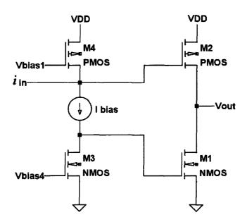
Figure 5.24 Push-pull output topology.
