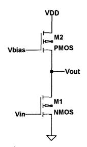
Figure 5.21 Common-source amplifier with a current source load.
