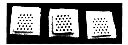
Figure 6.8 Master mold milled from Teflon stock.
