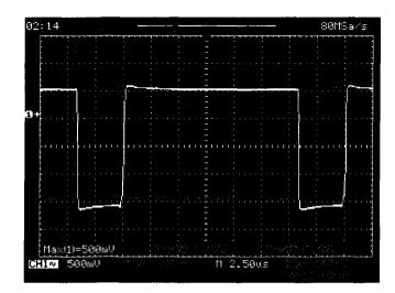
Figure 5.48 Inverted step response of one particular 250 fF amplifier.
