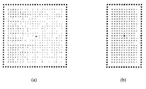
Figure 5 45 Capacitor layout for 500 (F(a) and 250 (F(b) capacitors
