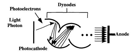
Figure 6.3 Dynode electron amplification.
