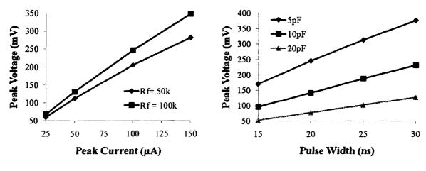
Figure 5.5 Peak output voltage with feedback capacitor of 5pF.
