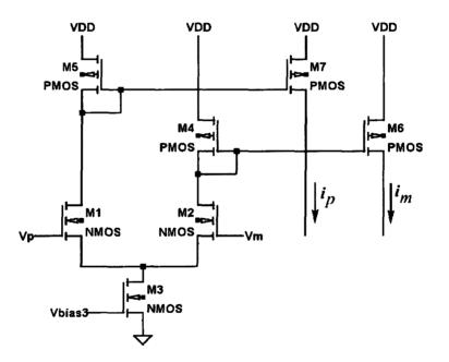
Figure 5.34 Comparator pre-amplification stage.
