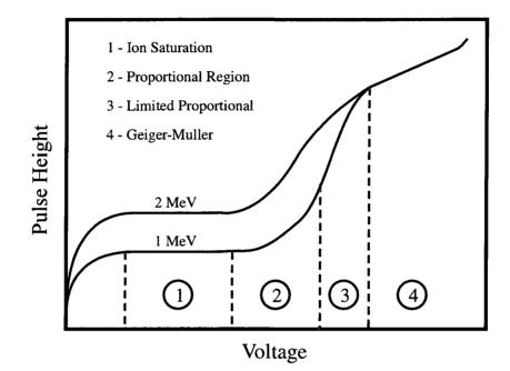
Figure 3.1 The different operating regions of gas-filled detectors.
