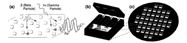
Figure 4.1 Glass and quartz substrates doped with boron nanoparticles converts radiation particles into optical pulses with varying heights which exit the scintillator (a). Optical pulses exiting the scintillator are directed away from the scintillating window by gold coated waveguides (b). The micro-device is patterned on-chip for a complete integrated radiation detection package (c).
