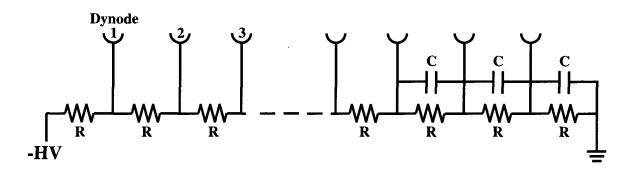
Figure 6.7 Schematic diagram of the voltage divider circuit.
