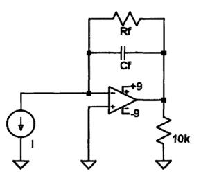
Figure 5.2 Schematic diagram of the simulated charge-sensitive preamplifier.
