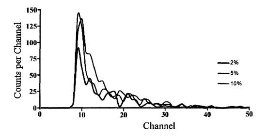
Figure 4.13 Energy spectrum of the quartz scintillator doped with 2%, 5% and 10% boron by weight.
