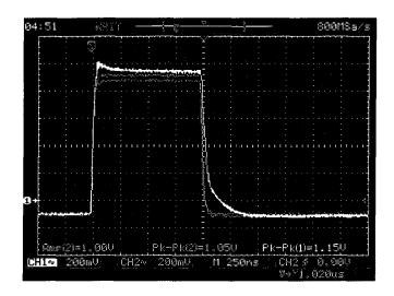
Figure 5.51 Step response of the 500 fF amplifier.
