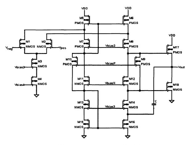
Figure 5.28 Two-stage operational amplifier design.
