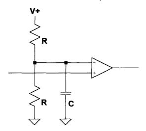
Figure 5.16 Comparator circuit used to trigger a microcontroller.
