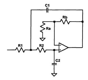
Figure 5.11 Schematic of a Sallen-Key low pass filter.
