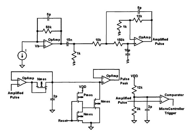
Figure 5.18 Radiation spectroscopy circuit for the integrated circuit layout.
