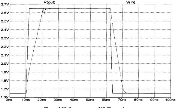
Figure 5.39 Step response, 500 fF capacitor.
