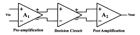
Figure 5.33 Block diagram of a comparator.
