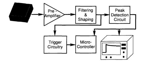
Figure 5.1 Block diagram of circuit components.
