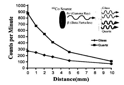
Figure 4.6 Quartz scintillator compared to the glass scintillator for beta detection.
