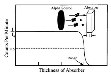
Figure 2.4 Range of alpha particles.
