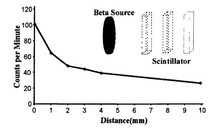
Figure 4.5 Beta counts verse distance for the glass scintillator.
