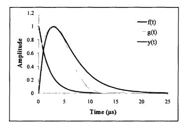
Figure 5.9 Preamplifier input and desired filter output.
