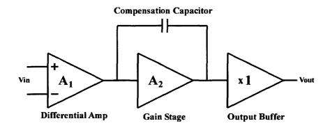
Figure 5.27 Two-stage operational amplifier block diagram.
