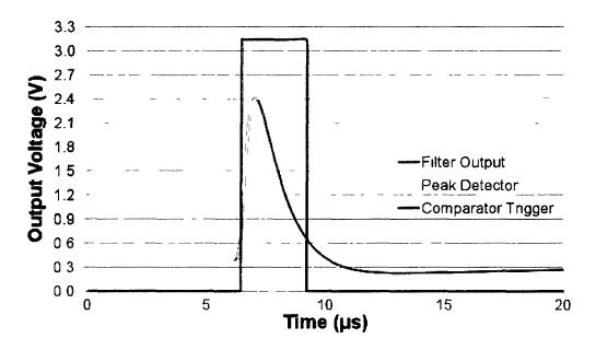
Figure 5.19 Output waveform of the radiation spectroscopy circuit.
