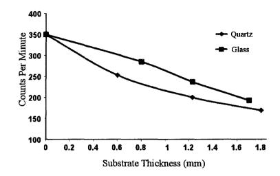
Figure 4.10 Glass and quartz absorption of gamma rays as substrate thickness is increased.
