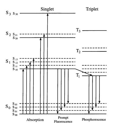
Figure 3.2 Configuration of organic scintillator electronic energy levels.
