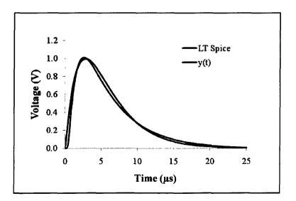
Figure 5.13 LT Spice simulation versus the desired output y(t).
