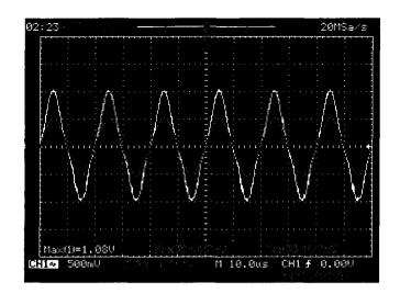
Figure 5.49 Non-inverted amplification of the 500 fF amplifier with a gain of two.
