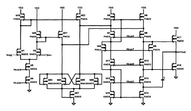
Figure 5.56 New comparator schematic.
