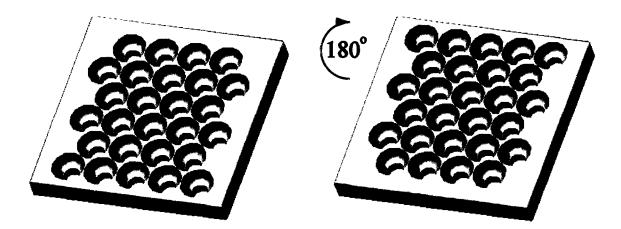
Figure 6.6 Second stack layer design; only a single layer is needed, requiring each layer to be rotated 180° as they are stacked.
