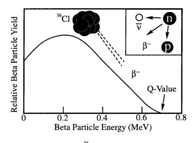
Figure 2.1 <sup>36</sup>Cl energy spectrum.
