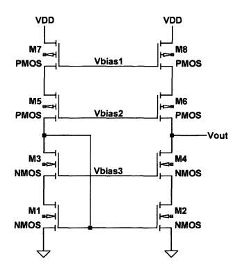
Figure 5.23 Folded cascode topology with diode connected pair.
