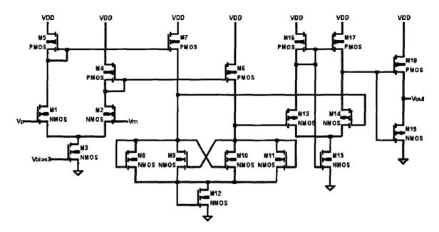
Figure 5.36 Comparator schematic.
