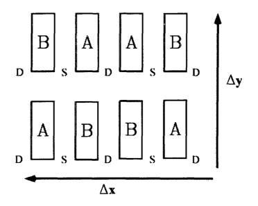
Figure 5.53 Common centroid layout of a transistor pair.
