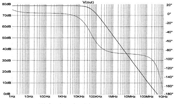
Figure 5.38 Open loop gain and phase response, 250 fF capacitor.
