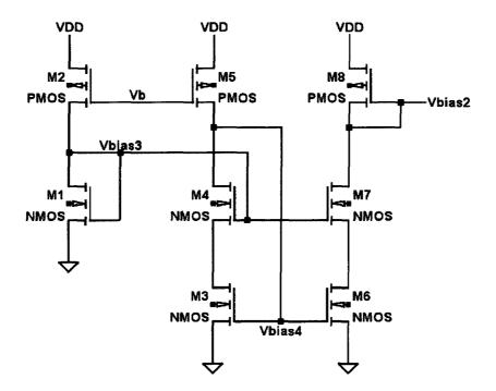
Figure 5.31 Current mirrors for bias voltages 2, 3, and 4.
