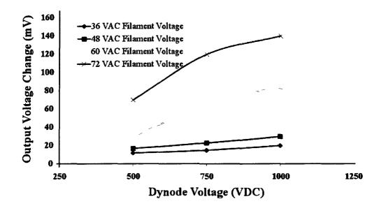
Figure 6.13 Voltage change versus dynode voltage for each filament voltage of the eight layer dynode stack.
