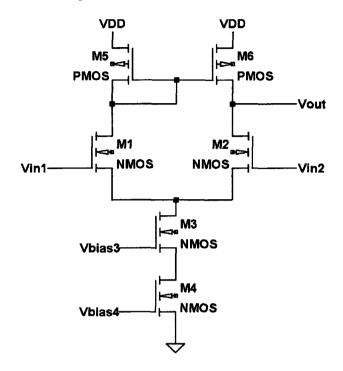
Figure 5.26 Differential amplifier with a current mirror load.
