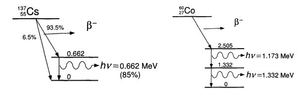
Figure 4.14 Decay scheme for cesium-137 and cobalt-60 radiation sources.
