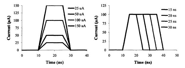
Figure 5.3 Varied input test currents with uniform pulse width.
