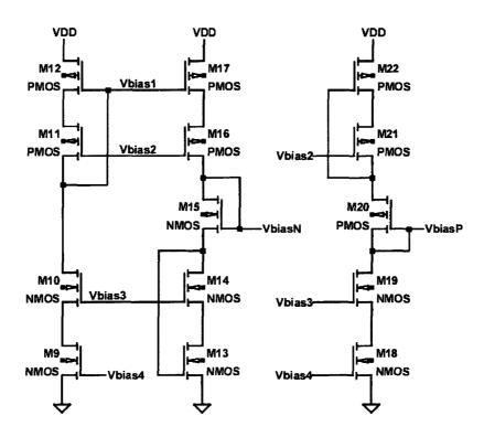
Figure 5.32 Current mirrors for bias voltages 1, N, and P.
