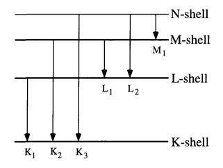
Figure 2.3 Possible electron orbital transitions.
