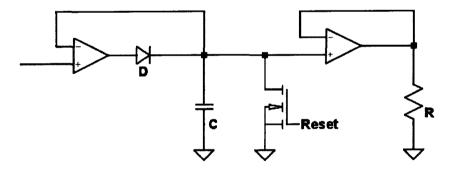
Figure 5.14 Schematic of a peak detector with op-amp buffers.
