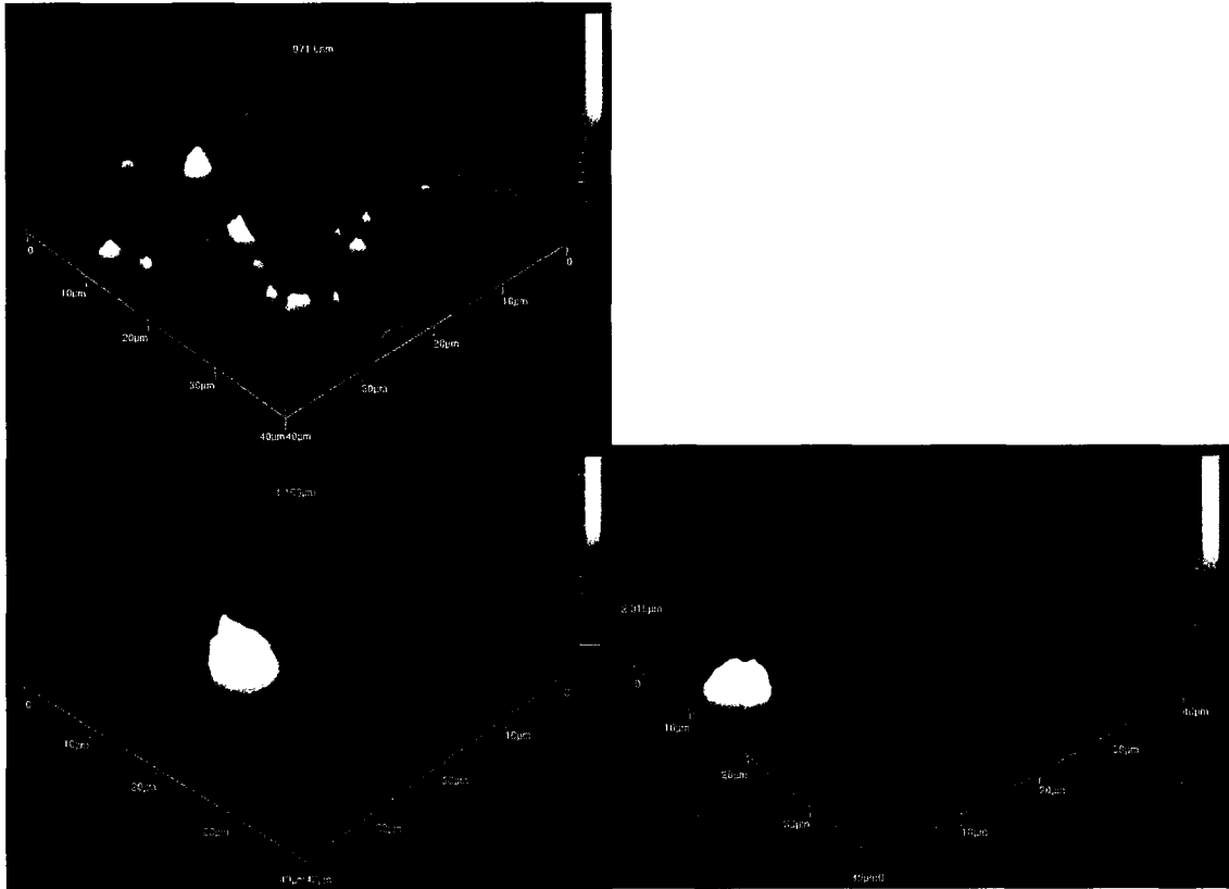
Figure 37 AFM images of slides with dLbL-collagen under static conditions (top left), and dynamic conditions at low (bottom left) and high shear (bottom right) exposed to plain PRP and stained with AO
