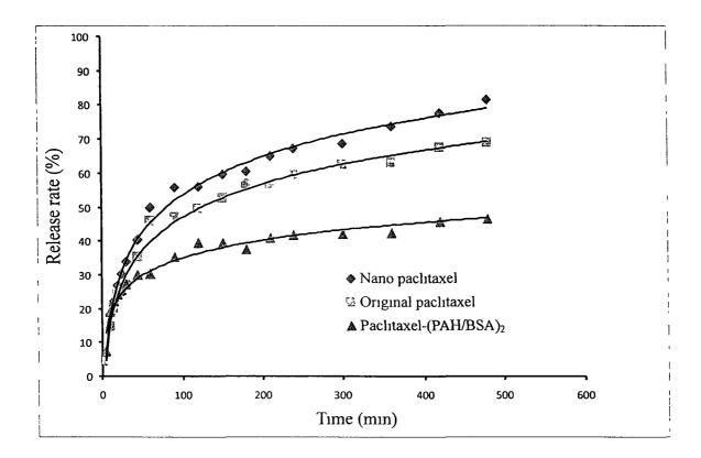
Figure 7-3 Release curves for the original micronized powder of paclitaxel, uncoated paclitaxel nanoparticles (only one PAH layer adsorbed for colloidal stabilization) and nano-encapsulated paclitaxel with (PAH/BSA)<sub>2</sub> shell composition
