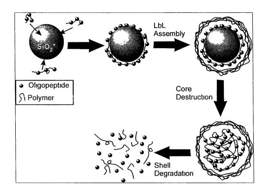
Figure 2-5 Degradable polymer microshells as carriers for the delivery of oligopeptide antigens
