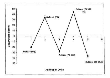
Figure 5-5 ξ-potential change during the LbL encapsulation of paclitaxel Standard deviation shows the same sample run 10 times on zeta potential analyzer
