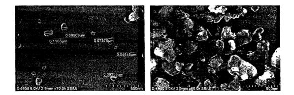
Figure 4-4 SEM image of the formed curcumin nanoparticles (left) diluted sample, and (right) concentrated sample
