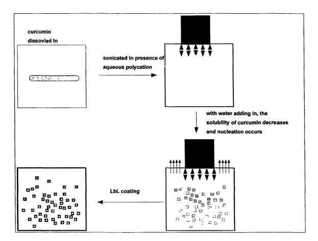
Figure 5-1 Scheme of the bottom-up curcumin LbL nanoformulation
