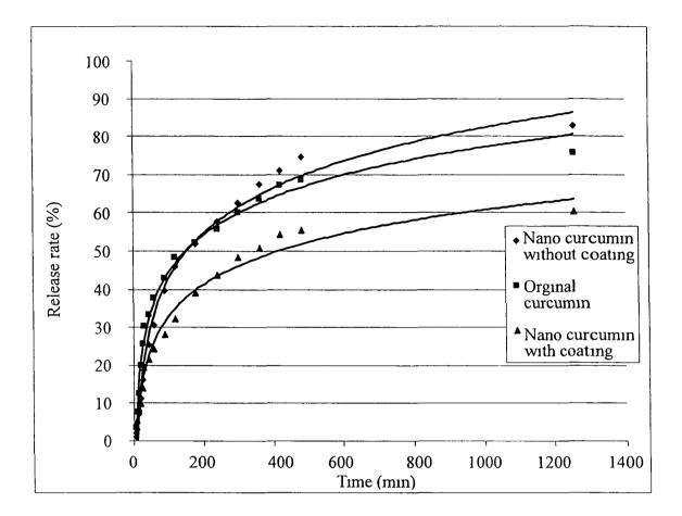
Figure 7-2 Release profiles of curcumin in original micropowder form, after nanoparticulation and prepared with LbL nano-encapsulation (the shell composition (PS/BSA)<sub>2</sub>)
