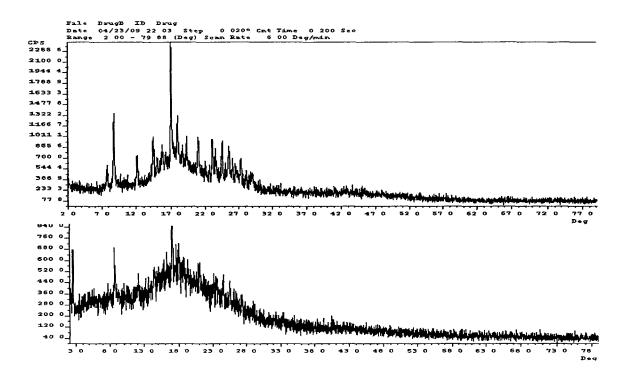
Figure 5-4 X-ray diffraction spectra for micronized curcumin powder (upper spectrum) and for nanoformulated curcumin (lower spectrum)
