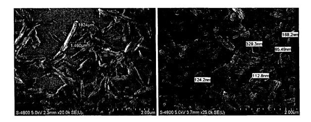
Figure 4-7 SEM image of orginal paclitaxel (left) and after ultrasound assisted LbL encapsulation with PAH/PSS/chitosan/alginic acid (right)
