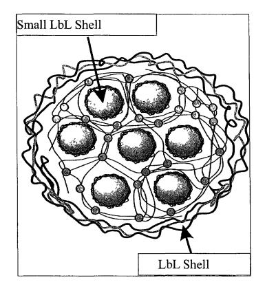
Figure 2-6 Self-exploding polyelectrolyte coated gel beads releasing micrometer-sized shells at the time of explosion
