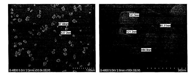
Figure 5-6 SEM image of paclitaxel nanoparticles with shells of (PS/PSA)<sub>2</sub> (left); same sample showing aggregation of particles at another site (right)
