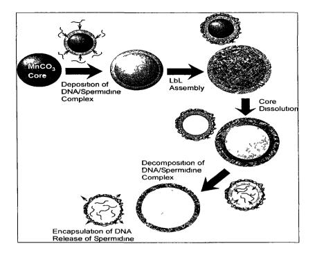
Figure 2-3 Preparation of functional hollow shells
