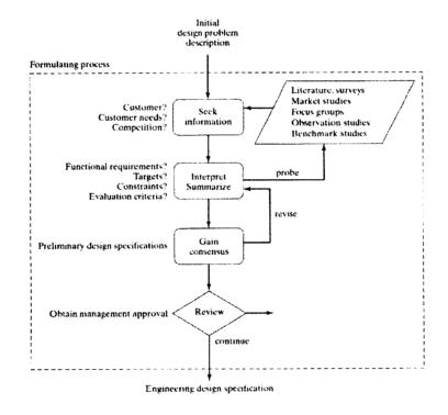
Figure 2-5: A flowchart identifying the formulation phase of the engineering design process [23].
