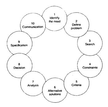
Figure 2-2: Illustration depicting the engineering design process as seen in the textbook *Engineering Fundamentals and Problem Solving* [24].
