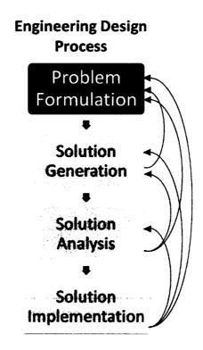
Figure 2-4: Illustration depicting a summarized version of the engineering design process.
