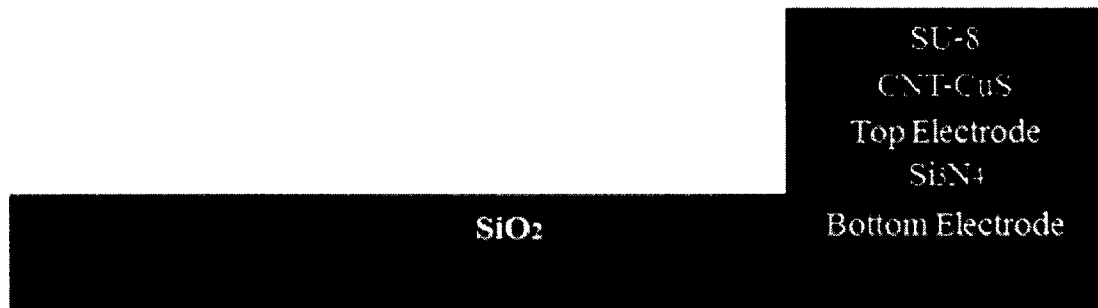
Figure 6-1 A thermoelectric generator with a thermal isolator ( \text{SiO}_2 ). Silicon and Au (red color) are used to form the generator. SWNTs-CuS thin film is used to enhance local temperature, and SU-8 layer is for protecting the thin film.
