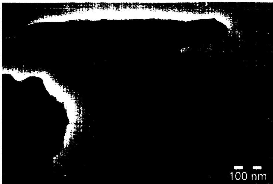
Figure 3- 9: TEM of barium coated halloysite nanotubes.
