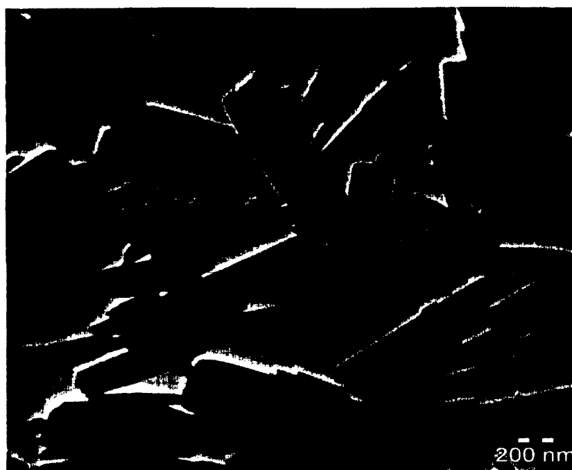
Figure 3- 3: TEM of control halloysite nanotubes.
