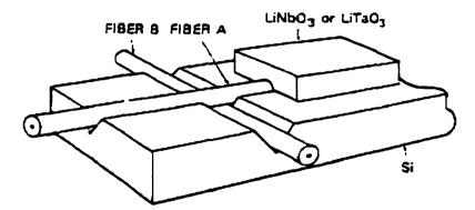
Figure 3-13. Fiber-to-Channel Waveguide Using Silicon Grooves [71]
