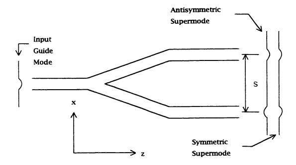
Figure 3-10. Characteristic Modes of a Symmetric Y-Junction [62]
