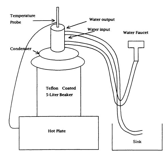
Figure 4-4 Anisotropic Etching System
