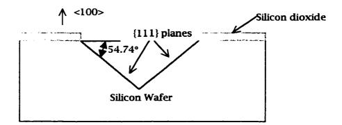
Figure 2-7. Micromachined Silicon Substrate
