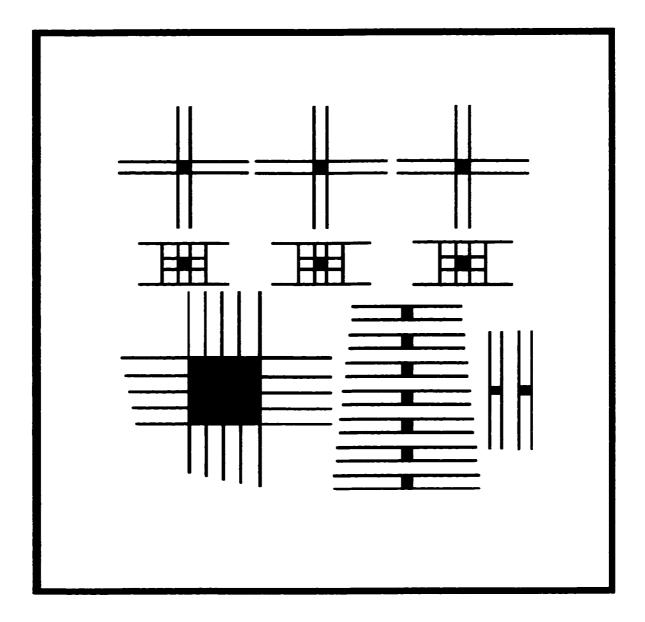
Figure 2-2. Mask Layer for Test Structures
