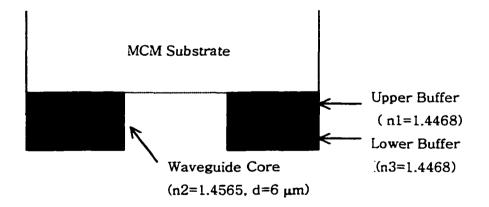
Figure 3-1. Silica Glass Waveguide Substrate
