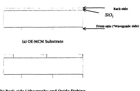
(b) Back-side Lithography and Oxide Etching
