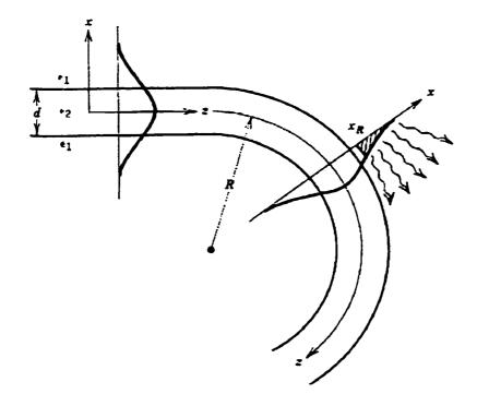
Figure 3-5. Bending Section of the Waveguide [58]
