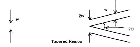
Figure 3-9. Y-Branching Waveguide Structure.
