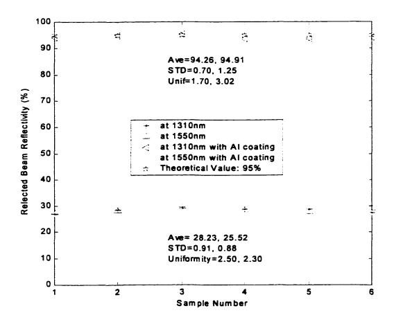
Figure 4-6. Beam Reflectivity of Silicon Mirror
