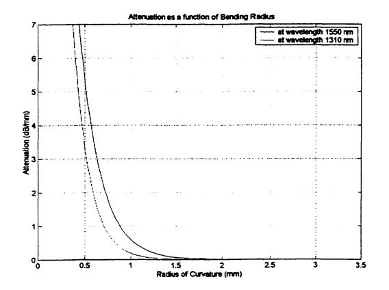
Figure 3-7. Attenuation as a Function of Bending Radius
