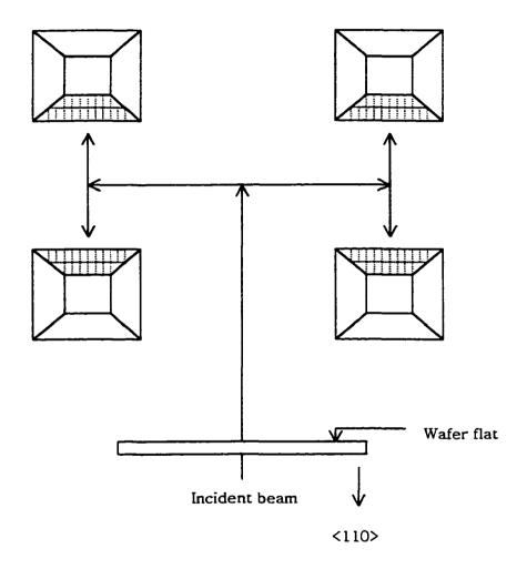
Figure 2-13. Direction of Incident Beam to 45° Mirrors
