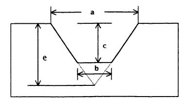
Figure 2-8. Geometry of an Etched Pit
