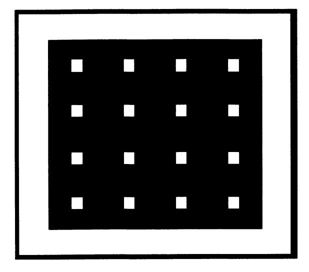
Figure 2-10. Mask Layer for Sixteen Through-Holes
