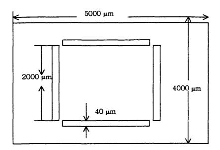
Figure 2-9. Mask Layer for Through-Holes
