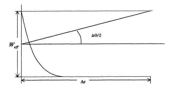
Figure 3-6. Radiation Aperture for Fields on a Curved Waveguide [58]
