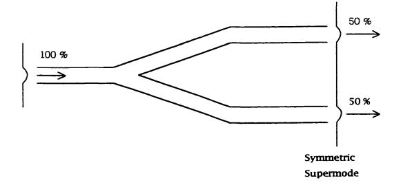
Figure 3-11. Excitation of a Y-Junction at the Left End [62]
