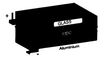
**Figure 4-5:** Basic layout of plasmonically enhanced photovoltaic device with SiO<sub>2</sub>/ITO/MDC/P3HT:PCBM/Al. Illumination is through a transparent electrode (ITO) with MDC on top of active layer.
