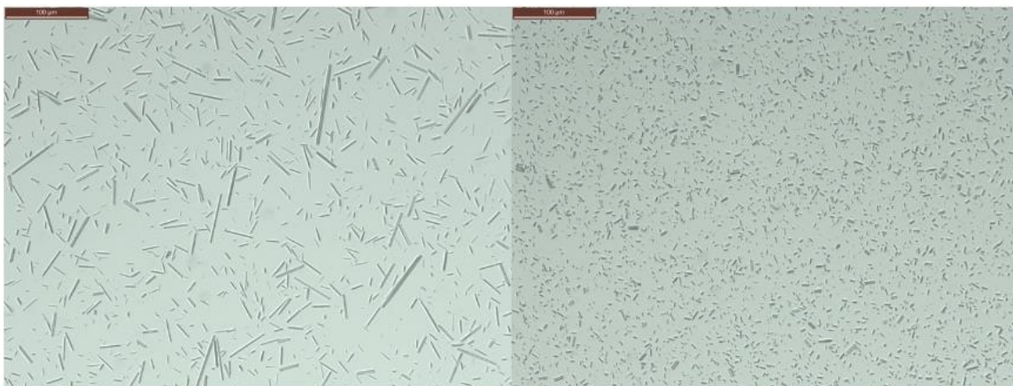
Figure 5.1: CuHARS before (left panel) and after (right panel) sonication. CuHARS were diluted to a final concentration of 10 \mu\text{g/ml} in sterile water. Pictures were taken using bright field microscope at 200x magnification. Scale bar = 100 \mu\text{m} .
