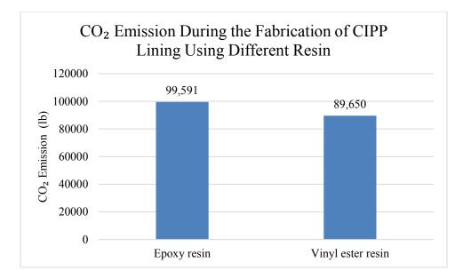
Figure 6-4 CO<sub>2</sub> Emissions During the Fabrication Phase for CIPP Lining Using Different Resin
