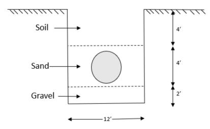
Figure 4-5 Pipeline Backfill Materials
