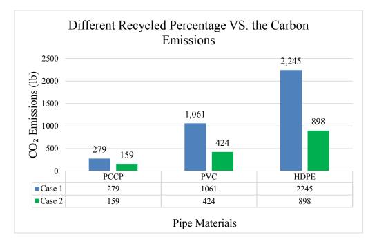
Figure 6-10 Different Recycled Percentage VS. the Carbon Emissions
