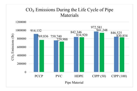
Figure 7-1 CO<sub>2</sub> Emissions During the Life-Cycle of Pipe Materials
