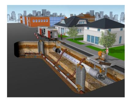
Figure 4-2 Schematic Diagram Shown the CIPP Installation Method (ISTT website)
