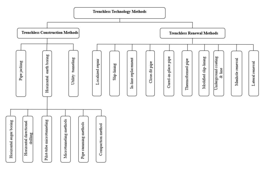
Figure 2-1 Pipeline Construction Methods (Trenchless Technology Methods)
