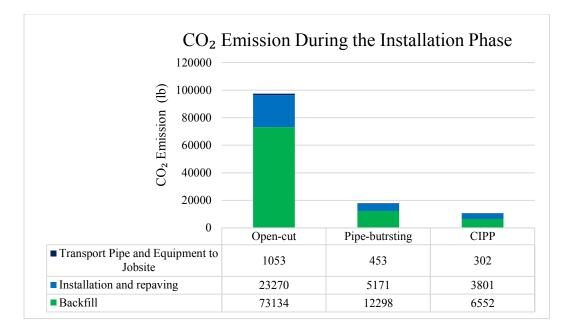
Figure 4-6 CO<sub>2</sub> Emissions During the Installation Phase
