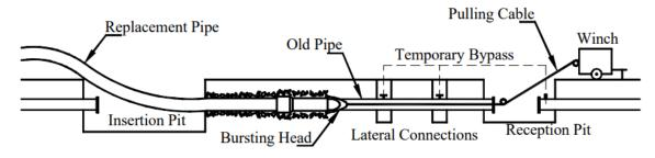
Figure 4-3 Pipe Bursting Operation Layout (TTC Report, 2001)
