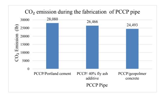
Figure 6-2 Comparing the CO<sub>2</sub> Emissions by Using Portland Cement, Fly Ash and Geopolymer Concrete During the Fabrication Phase of PCCP Pipe
