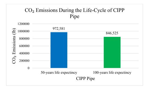
Figure 6-9 CO<sub>2</sub> Emissions During the 100 Years of Life-Cycle of CIPP Pipe
