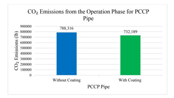
Figure 6-8 CO<sub>2</sub> Emissions During the Operation Phase of PCCP Pipe Before and After Coating
