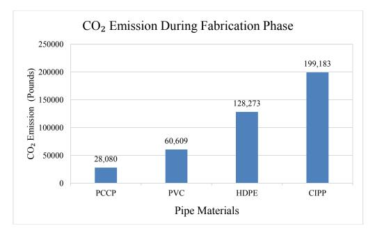
Figure 3-6 CO<sub>2</sub> Emission During the Fabrication Phase
