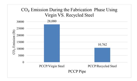
Figure 6-1 CO<sub>2</sub> Emissions During the Fabrication Phase for PCCP Pipe Using Virgin VS. Recycled Steel
