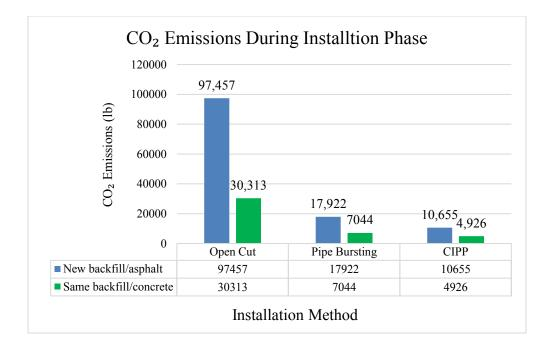
Figure 6-6 Comparing the CO<sub>2</sub> Emissions Between New Backfill Materials/Asphalt Pavement and Same Backfill Materials/ Concrete Pavement During the Installation Phase
