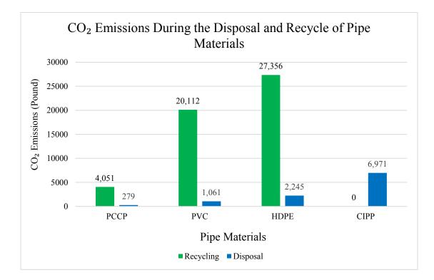
Figure 5-3 CO<sub>2</sub> Emissions During the Disposal Phase
