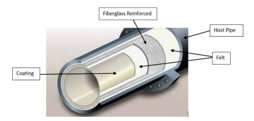
Figure 3-5 Schematic Cross Section for CIPP (http://www.premierpipeusa.com)
