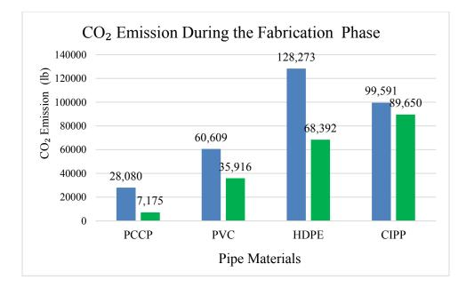
Figure 6-5 Shown the Difference Between the Pipeline Materials During the Fabrication Phase Before and After the Optimizing
