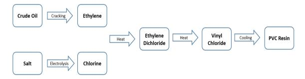
Figure 3-3 Cradle to Resin Flow Diagram of PVC Production (Krock, 2013)
