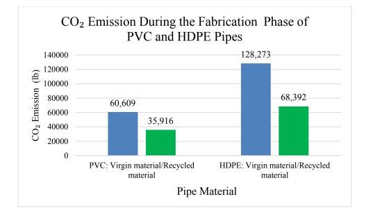
Figure 6-3 Comparing the CO<sub>2</sub> Emissions Between Virgin VS. Recycled Materials for PVC and HDPE Pipes
