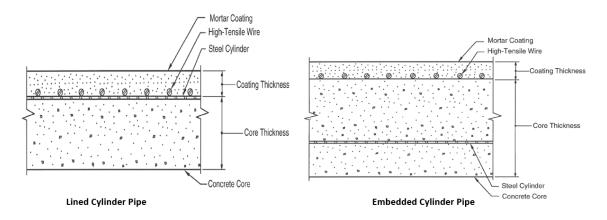
Figure 3-2 Schematic Shows the Different in Wall Cross Sections Between LCP and ECP Pipe (AWWA C304-14)
