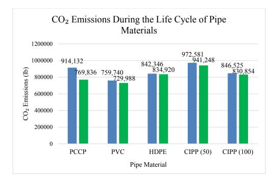
Figure 6-11 The Difference Between the Carbon Emissions During the Life-Cycle of Pipeline Materials Before and After Optimization, CIPP the First Two Columns are Presenting a 50-Years Life Expectancy, While the Last Two Columns are Presenting a 100-Years Life Expectancy
