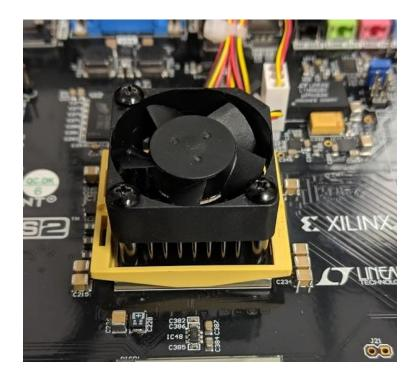
Figure 2-6: Stock forced-air cooling system for the Genesys 2 development board.
