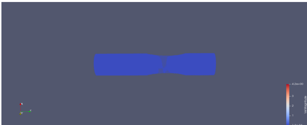
Figure 4-6: initial condition of the 25% cross-section stenosis blood vessel model.
