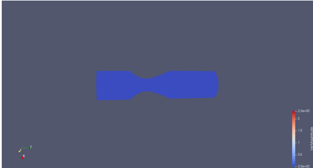
Figure 4-7: initial condition of the 75% cross-section stenosis blood vessel model.
