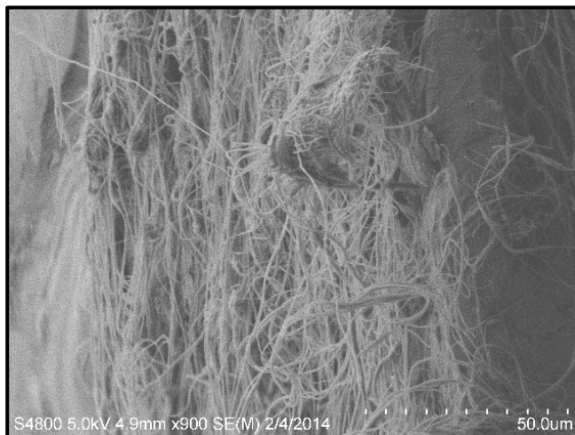
Figure 3-3: Pre-calcination disordered nanofibers.
