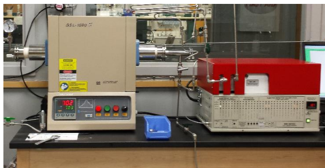
Figure 3-10: Thermal plug flow reactor (GSL-1500X MTI Corp.) with in-line GC (SRI 8610C, SRI Corp).
