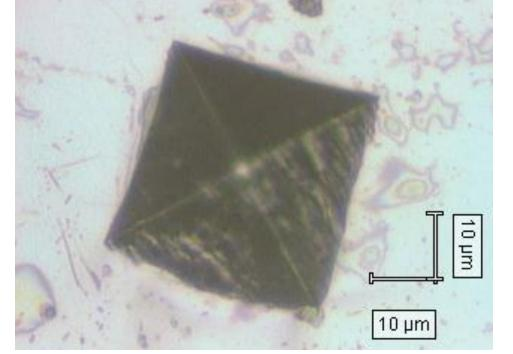
In an attempt to simulate natural defects, artificial pits were manufactured using a diamond tip. Regular indentations were made on the surface of a Niobium foil.
