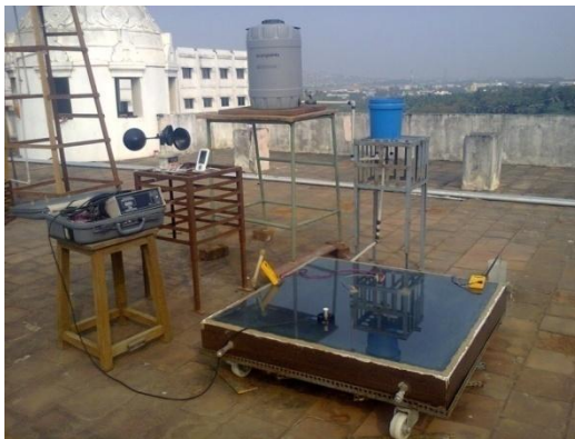
Fig. 3. Photograph of the shallow solar pond with 6cm depth
