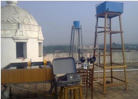
Fig. 4. Photograph of the shallow solar pond with 15cm depth
