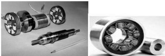
Gambar 1. Active Magnetic Bearing
