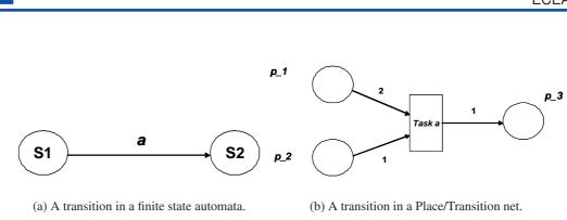
Figure 3: Examples of transition systems modelled by WIPPOGrules.
