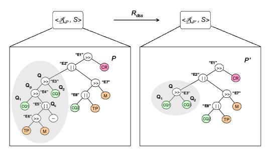
Figure 8: Process Transformation 1: Sequence Delete in Sequence Construct.
