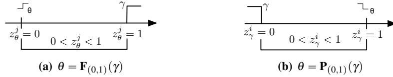
Figure 2: Depiction of some conditions for raising and falling edges in metric operators.
