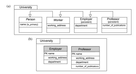
Figure 2: The UML model (a) and the correspondent RDBMS model (b)
