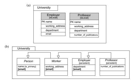
Figure 3: The modified RDBMS model (a) and the correspondent UML model (b)
