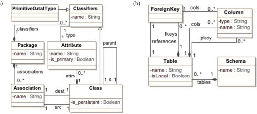
Figure 1: Simplified UML (a) and RDBMS (b) metamodels
