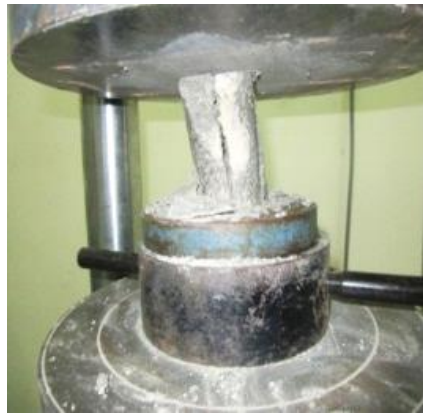
Figure 14. Grouted sand failure.
