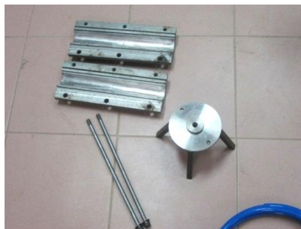
Figure 7. Mould for sand sample.
