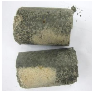
Figure 13. Grouted sand samples.
