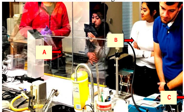
Fig.4. On running the Bi-Polar ® unit the smoke in the fiber glass chamber was gone in 60 seconds. Cigarette smoke was inserted into a fiber glass chamber through an inlet while a Bi-Polar ® unit was running inside. The stop watch showed the time for reduction of the smoke concentration. The video recording of the experiment showed a complete reduction of smoke in the fiber glass chamber. The video is available on the YouTube with a link: https://www.youtube.com/watch?v=LpB6qZv0n_M (Ref. Bennert, J, 2016).
