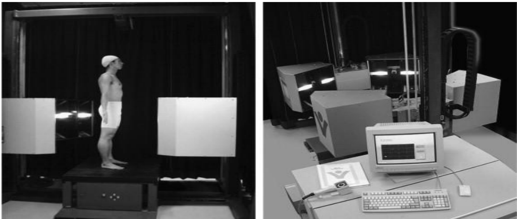
Figure 4. Vitus 3-D 1600 whole body scanning system (Lu and Wang, 2008).
