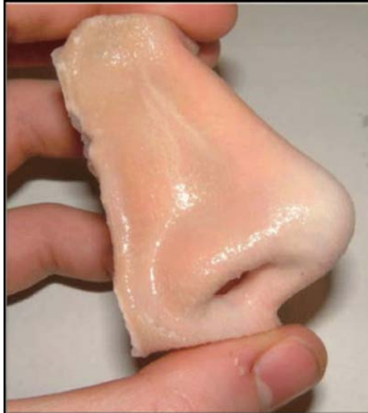
Figure 1: Photograph of a silicone infiltrated 3D printed powdered construct used to manufacture a bespoke nasal soft tissue prosthesis. Geometry and colour data were translated throughout the CAD/CAM design and manufacturing process.
