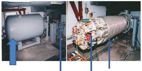
Tank Switching magnet Electronics Accelerator Tube
