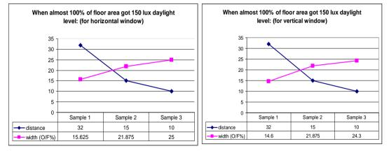
From the figure above it is revealed that required opening, floor area and window ratio for target daylight level is **inversely proportionate** with building-to-building distance for both horizontal and vertical opening
