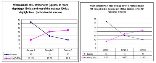
From the figure above it is revealed that required opening, floor area and window ratio for target daylight level is **inversely proportionate** with building-to-building distance for different amount of daylight inclusion.
