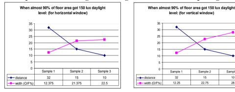
From the figure it is revealed that required opening, floor area and and window ratio for target daylight level is inversely proportionate with building to building distance for both horizontal and vertical opening.
