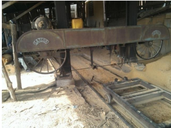
Figure 4: Typical example of squaring machine in Lomé in 2014
