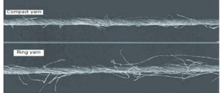
Figure 1: Yarn structure of compact yarn and conventional ring spun yarn (microscopic view) ( Lawrence, 2010, 240).
