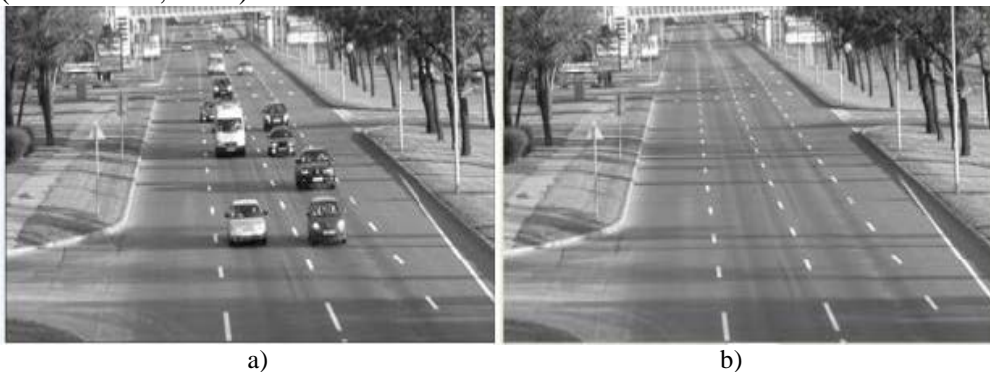
Fig 1. The initial frame (a) and static background obtained by temporal filtering (b)
