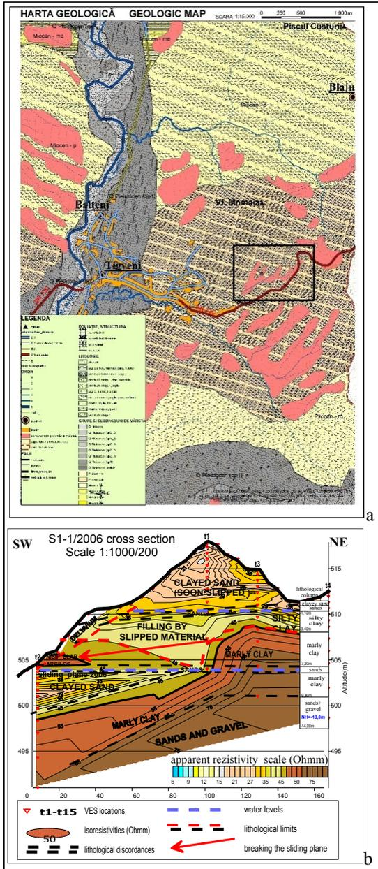
Geological settings, in surface and in depth reveal the lithological and structural peculiarity of landslides. Mapping rock strata, types of natural deposits and fillings, thickness and spatial variation, the method is interposed between morphological surface mapping and geotechnical data analysis and geophysical research.
