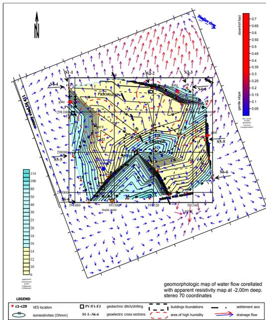
Slips developed subsequent layer perpendicular to the surface and in conditions of favorable hydro-geological parameters they either can have a tendency to stretch and asymmetric upstream side or often can be reactivated in case of cracks lithology less resistant layers (Balteni) (Fig 8b.). The obsequent landslides develop on the heads of lithological strata and have more roughness morphology.
