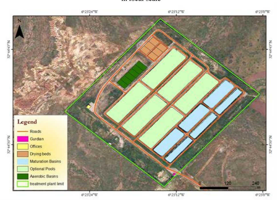
Figure 2. Various structures of the Boujaad Wastewater Treatment Plant
