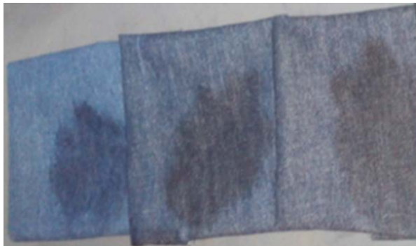
Figure 15. Photographic view of chlorine bleached samples after water repellency test
