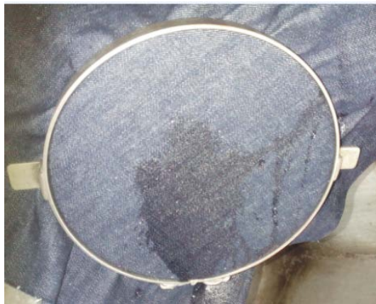
Figure 14. Photographic view of raw sample after water repellency test
